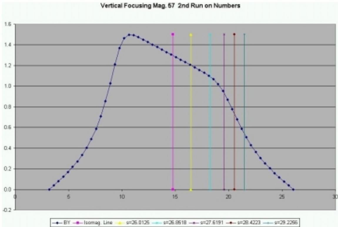
Figure 1. This chart is an illustration of the B<sub>y</sub> field graphed vs. the distance through the magnet. On this chart is the isomagnetic line and the beam trajectory displacement at ends of the 4 pieces this magnet was partitioned into. The isomagnetic line is the vertical line to the far left. The line to the right of that is the beginning of the pieces the magnets were cut into. The far right vertical line represents the end of the last piece.
