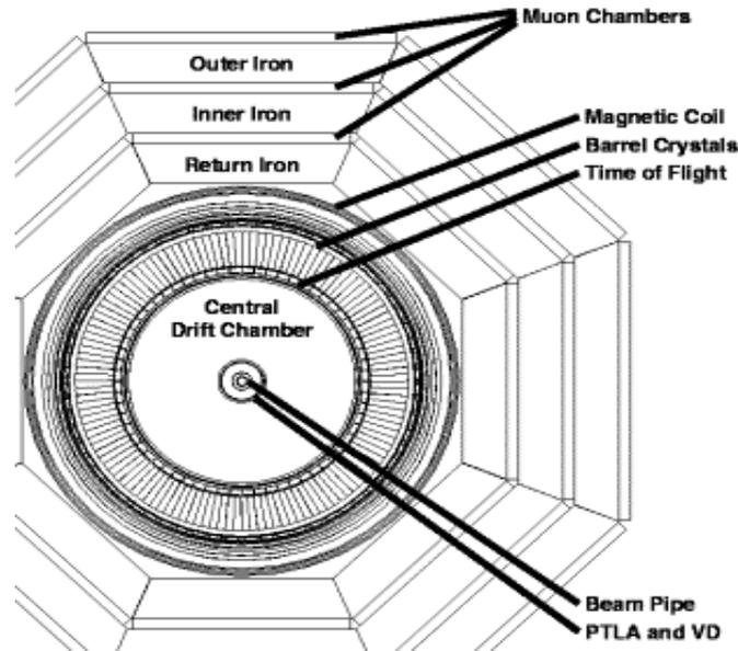
**FIGURE 2** CLEO II detector. The elements of primary concern are the drift chamber and the barrel crystals (crystal calorimeter).
