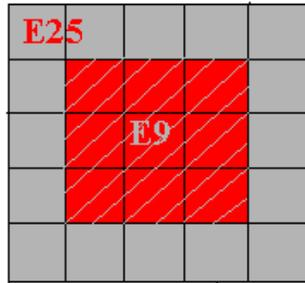
**FIGURE 8** A representation of a twenty-five crystal block in the crystal calorimeter.
