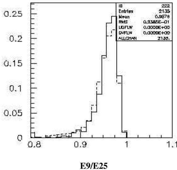
**FIGURE 9** A normalized plot of E9/E25. Though its peak is close to one, there remains a large tail. The expected is the dashed line and the experimental, solid.
