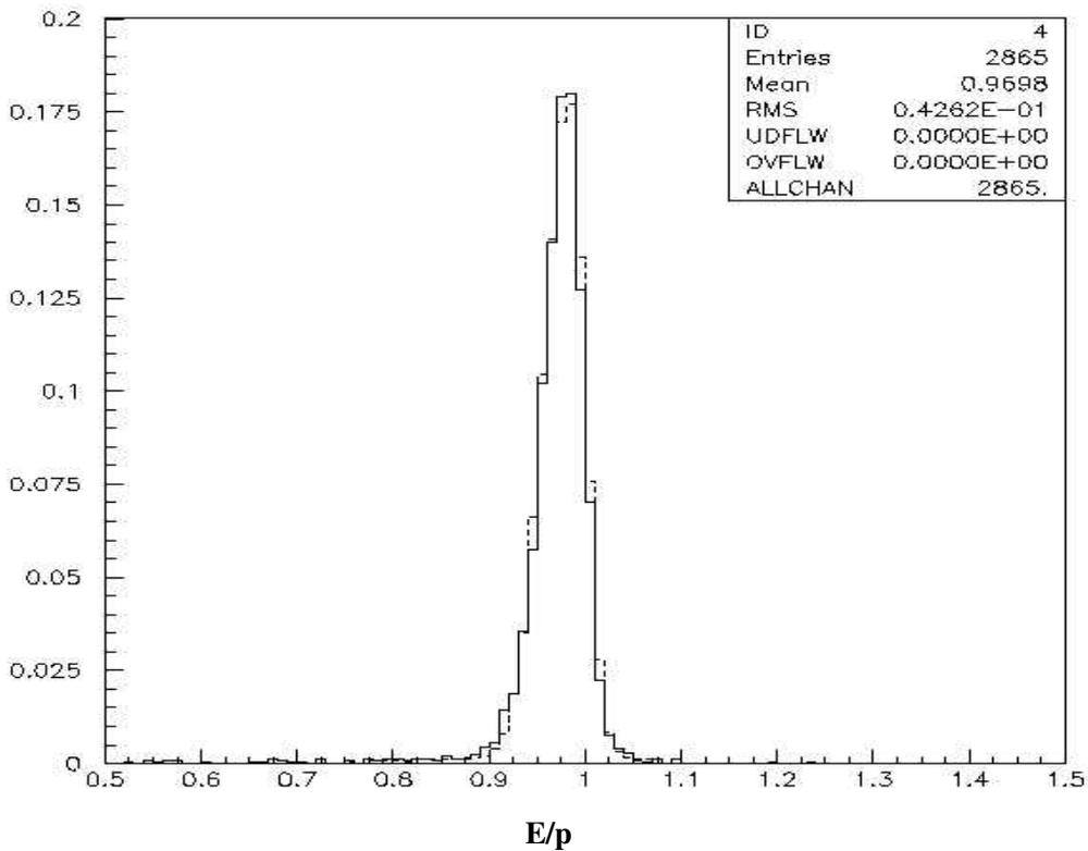
**FIGURE 6** A graph of  $E/p$  normalized to see the relation of the code's prediction (dashed line) and the experimental results from looking at clean radiative bhabha samples.
