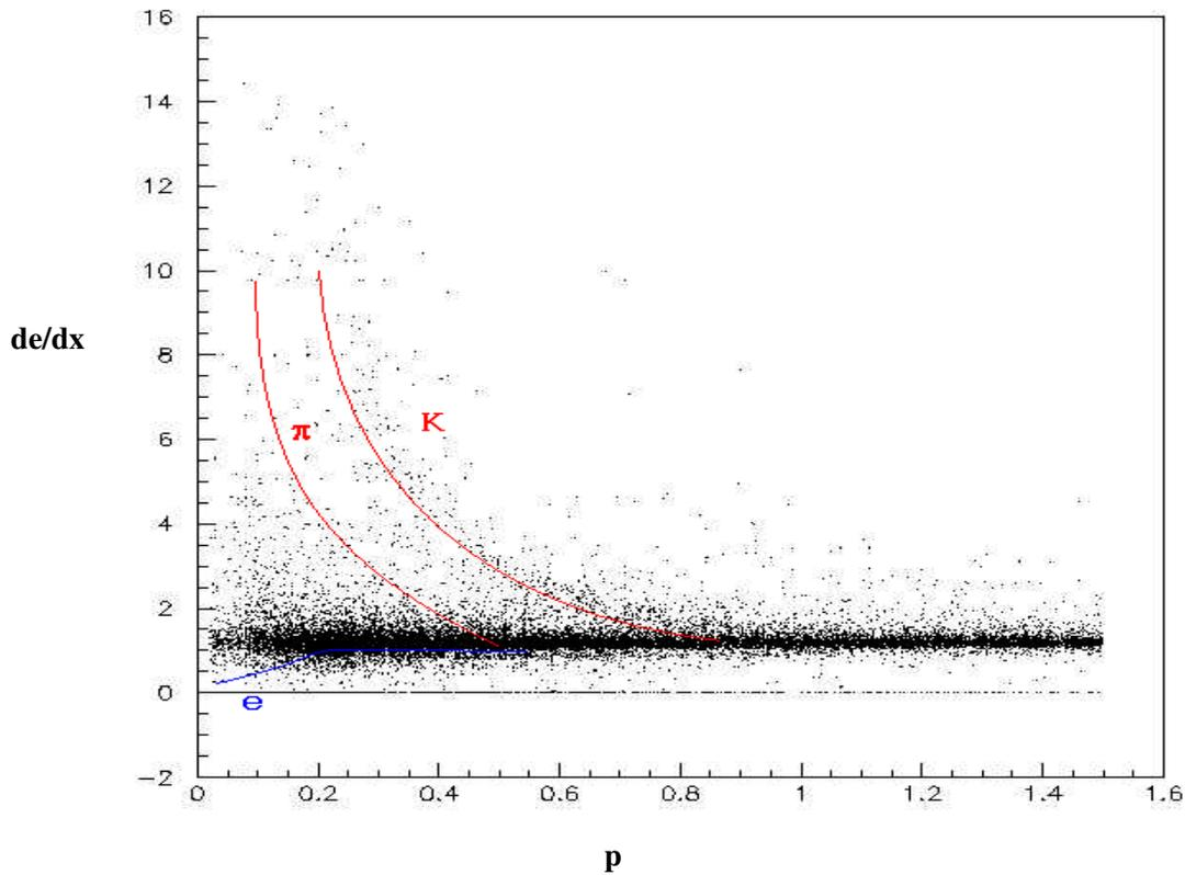
**FIGURE 7** A graph of  $de/dx$  versus momentum. As momentum increases, the various  $de/dx$  measurement converge. The colored lines have been sketched in to show the approximate location and shape of a particle's  $de/dx$  plot.
