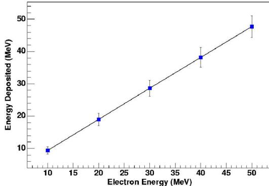
FIG. 3: Results of GEANT4 simulations of energy deposited in a  $20 \times 30 \times 30$  cm CsI scintillator. Energy deposited is compared to electron energy upon entering the scintillator. This plot illustrates that the scintillator can measure electron energy to within 3 MeV.
