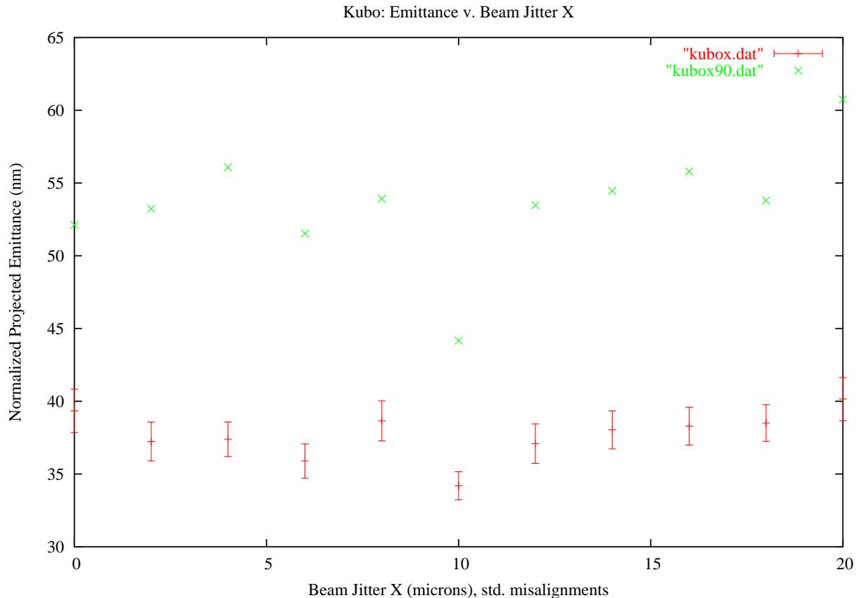
FIG. 3: Kubo with x-Beam Jitter and Standard Misalignments - “kubox.dat” represents the mean emittance of 100 seeds with the error bars (where error is the ratio of standard deviation to the square root of the number of seeds). “kubox90.dat” represents the 90 percent confidence level
