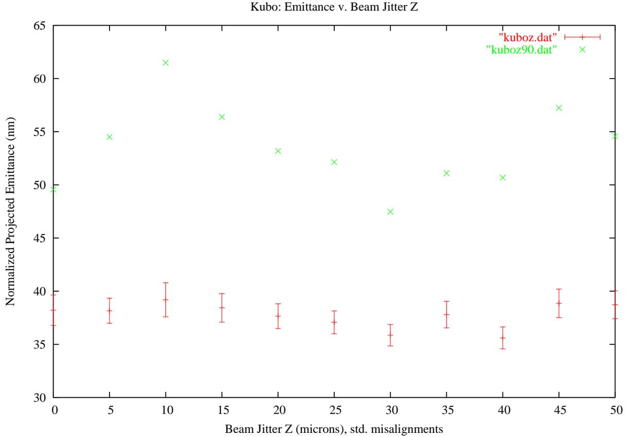
FIG. 9: Kubo with z-Beam Jitter and Standard Misalignments - “kuboz.dat” represents the mean emittance of 100 seeds with the y error bars (where error is the ratio of standard deviation to the square root of the number of seeds). “kuboz90.dat” represents the 90 percent confidence level
