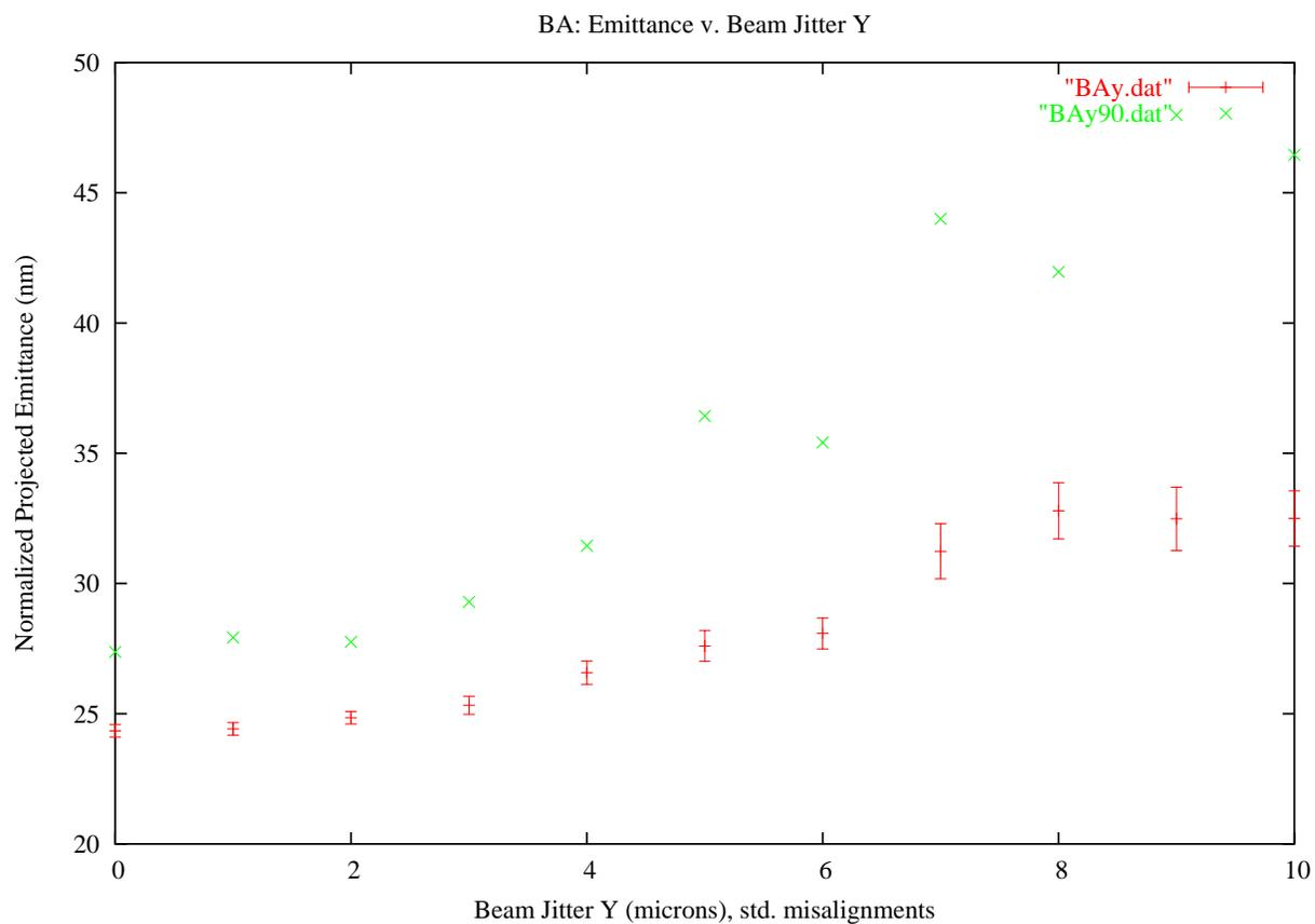
FIG. 4: Ballistic Alignment with y-Beam Jitter and Standard Misalignments - “bay.dat” represents the mean emittance of 100 seeds with the error bars (where y error is the ratio of standard deviation to the square root of the number of seeds). “bay90.dat” represents the 90 percent confidence level
