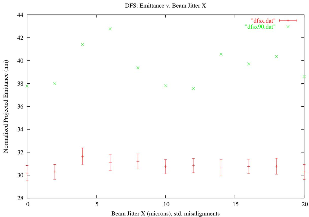
FIG. 2: DFS with x-Beam Jitter and Standard Misalignments - “dfsx.dat” represents the mean emittance of 100 seeds with the error bars (where error is the ratio of standard deviation to the square root of the number of seeds). “dfsx90.dat” represents the 90 percent confidence level
