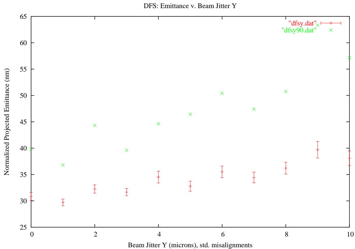
FIG. 5: DFS with y-Beam Jitter and Standard Misalignments - “dfsy.dat” represents the mean emittance of 100 seeds with the error bars (where error is the ratio of standard deviation to the square root of the number of seeds). “dfsy90.dat” represents the 90 percent confidence level
