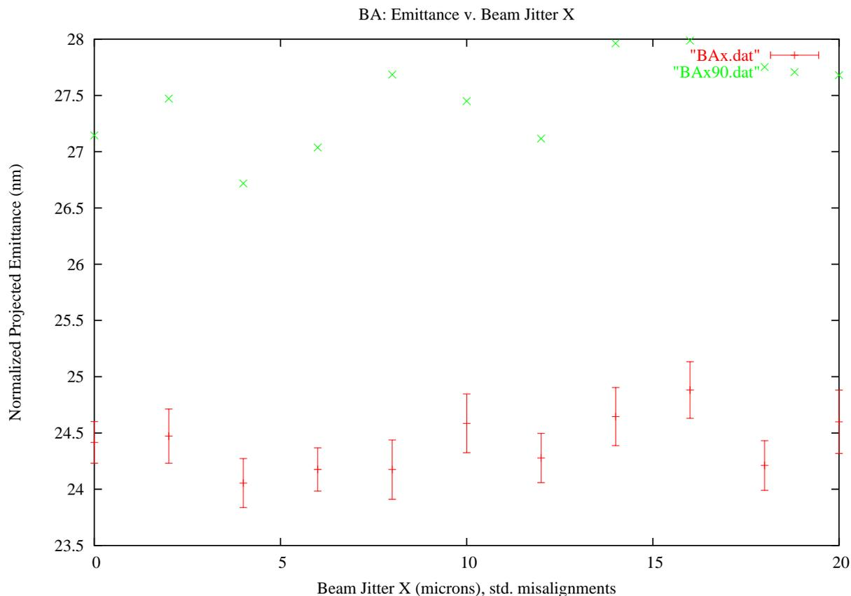
FIG. 1: Ballistic Alignment with x-Beam Jitter and Standard Misalignments - “bax.dat” represents the mean emittance of 100 seeds with the error bars (where y error is the ratio of standard deviation to the square root of the number of seeds). “bax90.dat” represents the 90 percent confidence level. Note that even at twenty micron jitter even the ninety percent confidence value of emittance is still below 40 nm allowance.
