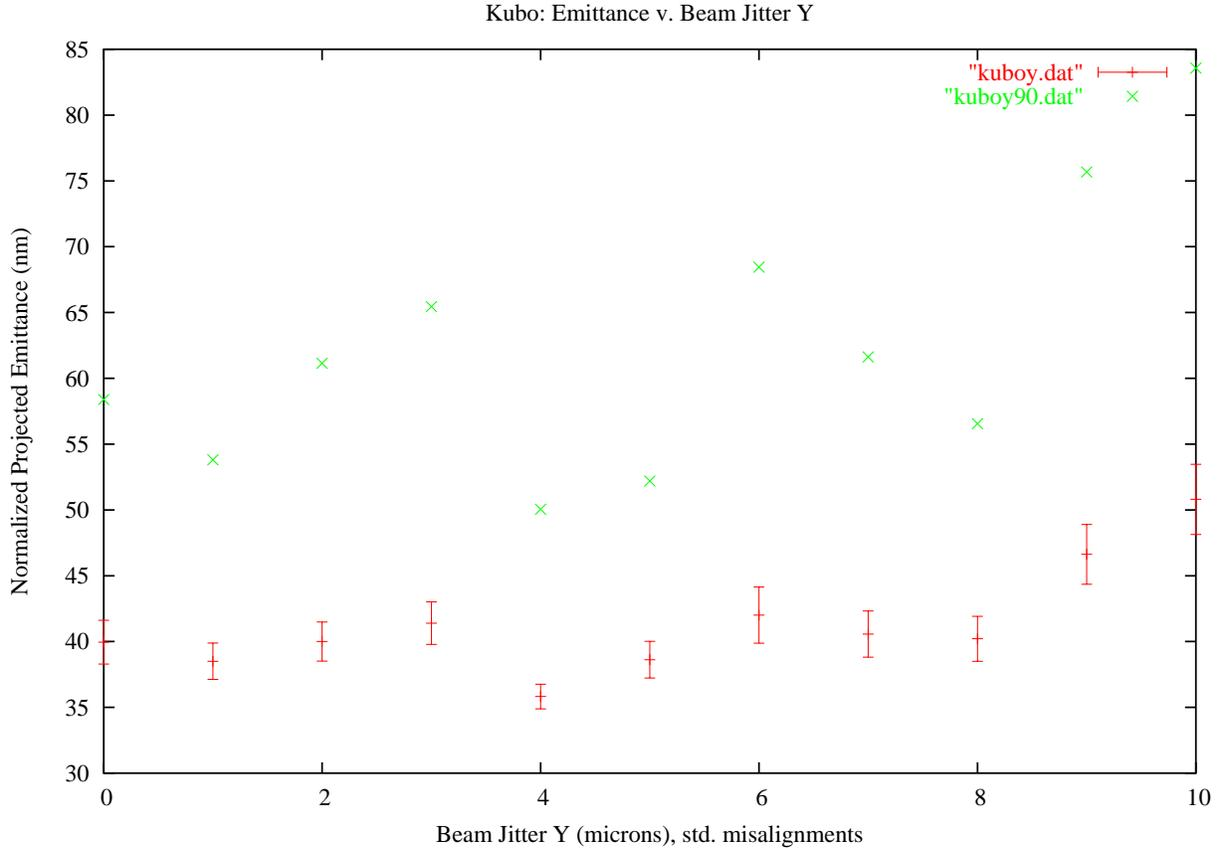
FIG. 6: Kubo with y-Beam Jitter and Standard Misalignments - “kuboy.dat” represents the mean emittance of 100 seeds with the y error bars (where error is the ratio of standard deviation to the square root of the number of seeds). “kuboy90.dat” represents the 90 percent confidence level
