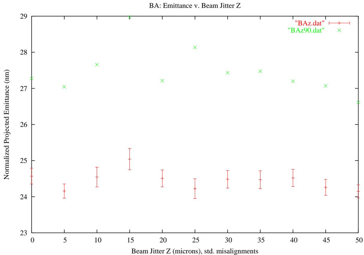
FIG. 7: Ballistic Alignment with z-Beam Jitter and Standard Misalignments - “BAy.dat” represents the mean emittance of 100 seeds with the y error bars (where error is the ratio of standard deviation to the square root of the number of seeds). “BAy90.dat” represents the 90 percent confidence level
