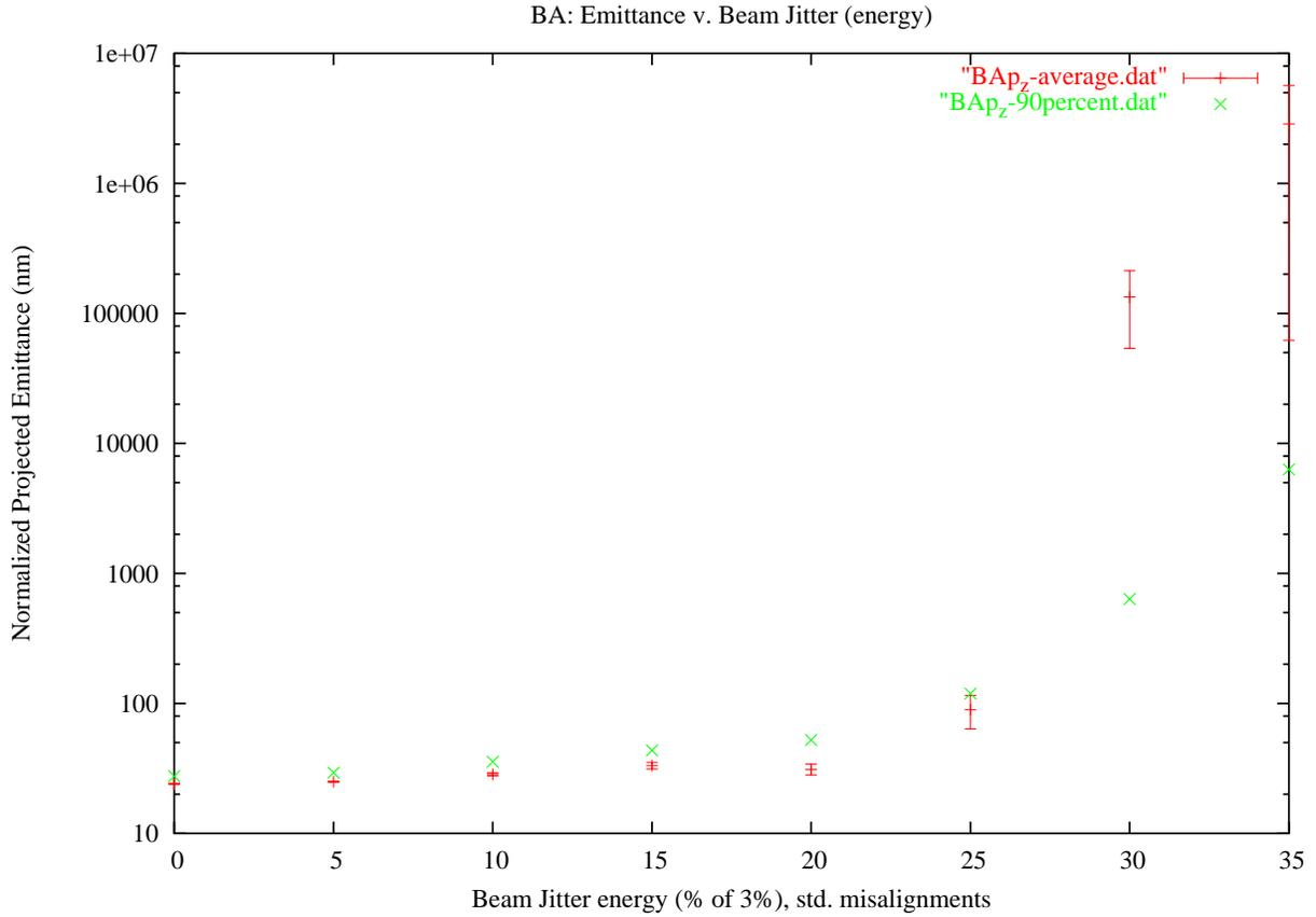
FIG. 10: Ballistic Alignment with  $z'$  Beam Jitter and Standard Misalignments-“ $BAp_z - average.dat$ ” represents the mean emittance of 100 seeds with the error bars (where error is the ratio of standard deviation to the square root of the number of seeds). “ $BAp_z - 90percent.dat$ ” represents the ninety percent confidence level.
