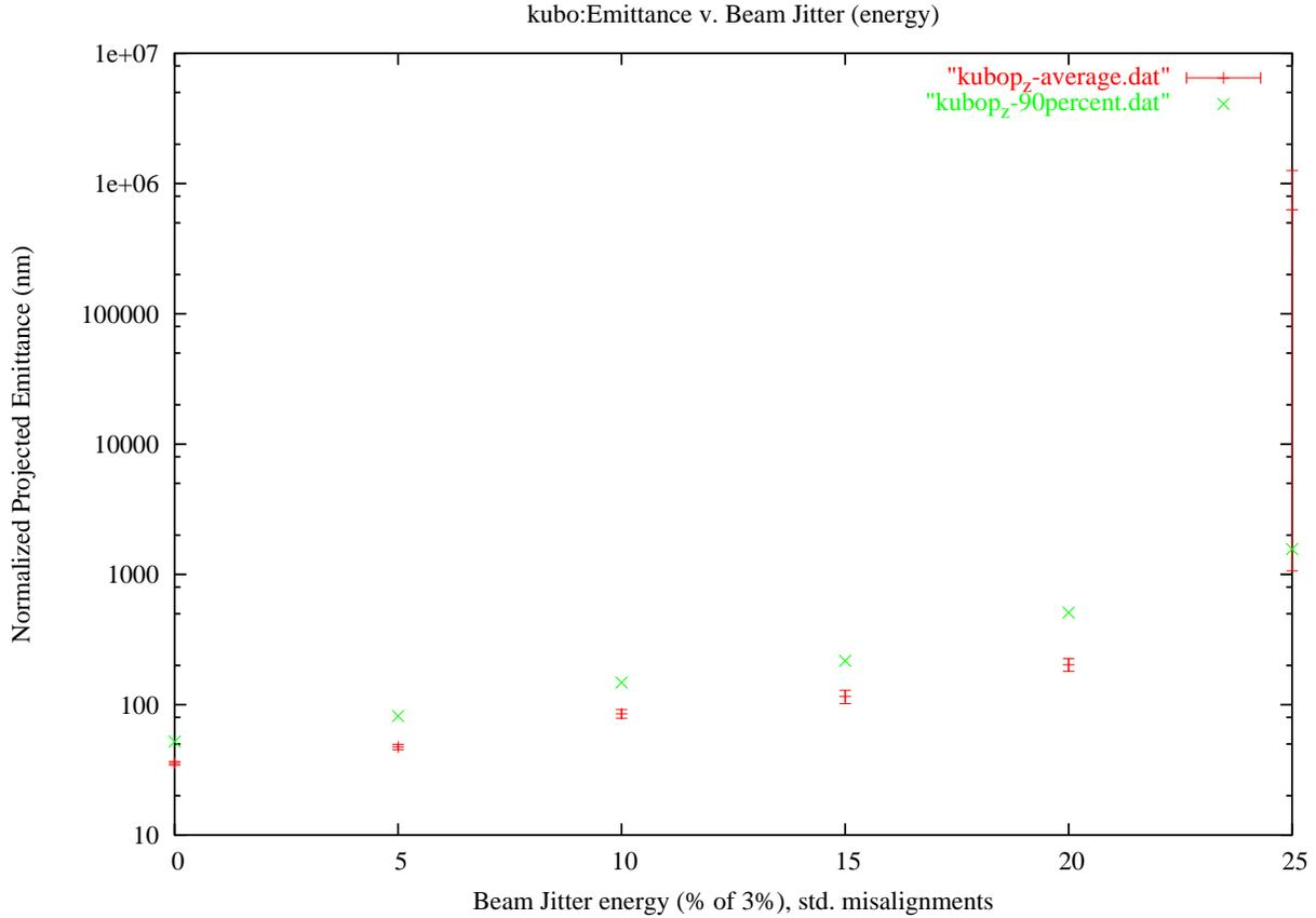
FIG. 12: Kubo with  $z'$  Beam Jitter and Standard Misalignments-“ $kubop_z - average.dat$ ” represents the mean emittance of 100 seeds with the error bars (where error is the ratio of standard deviation to the square root of the number of seeds). “ $kubop_z - 90percent.dat$ ” represents the ninety percent confidence level.
