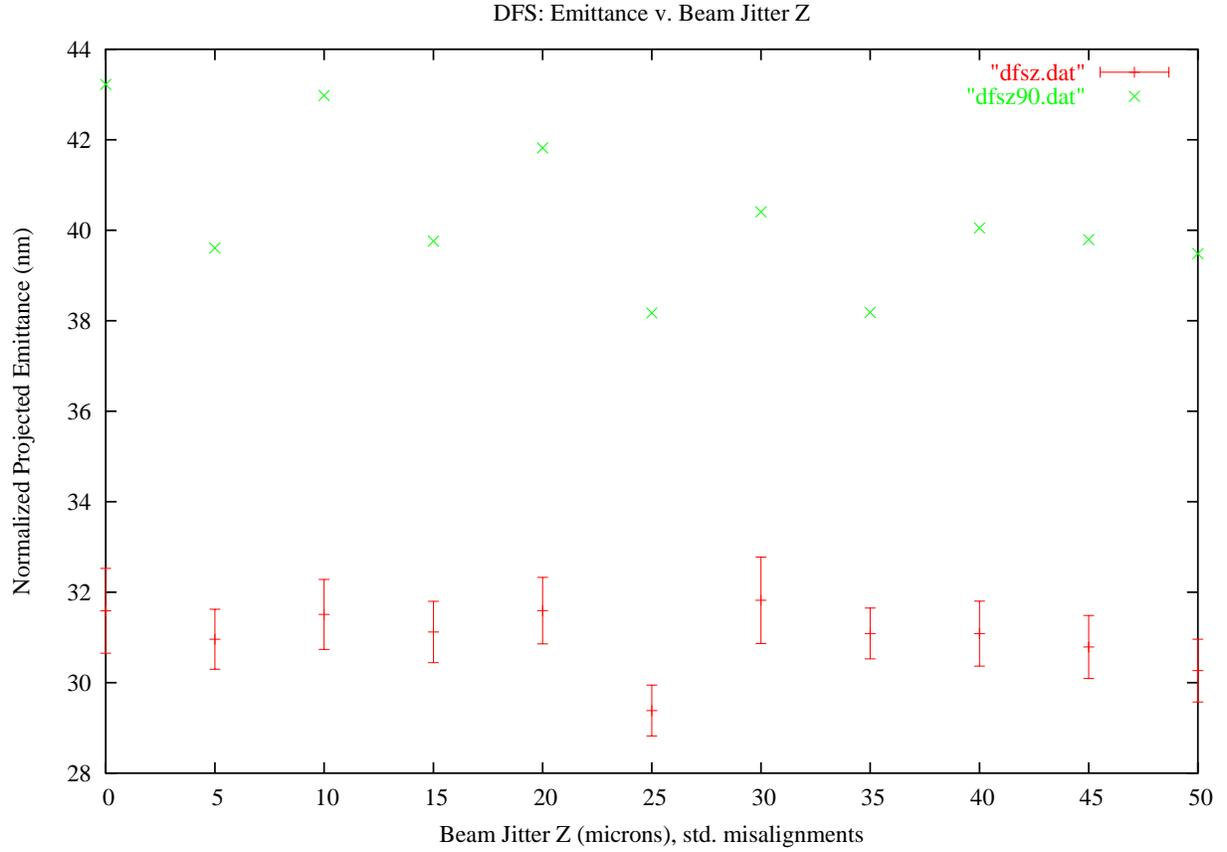
FIG. 8: DFS with z-Beam Jitter and Standard Misalignments - “dfs.sz.dat” represents the mean emittance of 100 seeds with the y error bars (where error is the ratio of standard deviation to the square root of the number of seeds). “dfs.sz90.dat” represents the 90 percent confidence level
