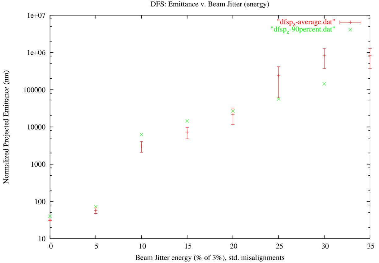
FIG. 11: DFS with  $z'$  Beam Jitter and Standard Misalignments-“ $dfsp_z - average.dat$ ” represents the mean emittance of 100 seeds with the error bars (where error is the ratio of standard deviation to the square root of the number of seeds). “ $dfsp_z - 90percent.dat$ ” represents the ninety percent confidence level.
