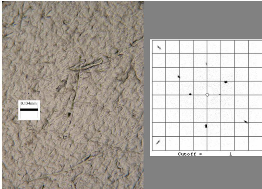
FIG. 9: non heat affected zone after the EBW process with back reflection Laue pattern
