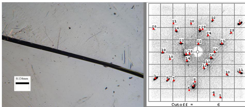
FIG. 2: sample 1 after 900 C heat treatment for 1 hour with known grain boundary, back reflection Laue method pattern taken from above grain boundary
