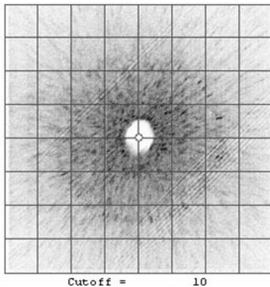
FIG. 12: back reflection Laue pattern of a known poly crystal
