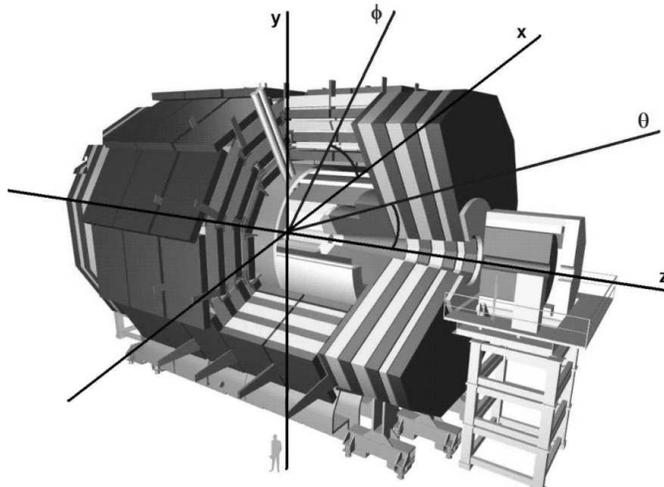
FIG. 2: Coordinates for the CMS detector
