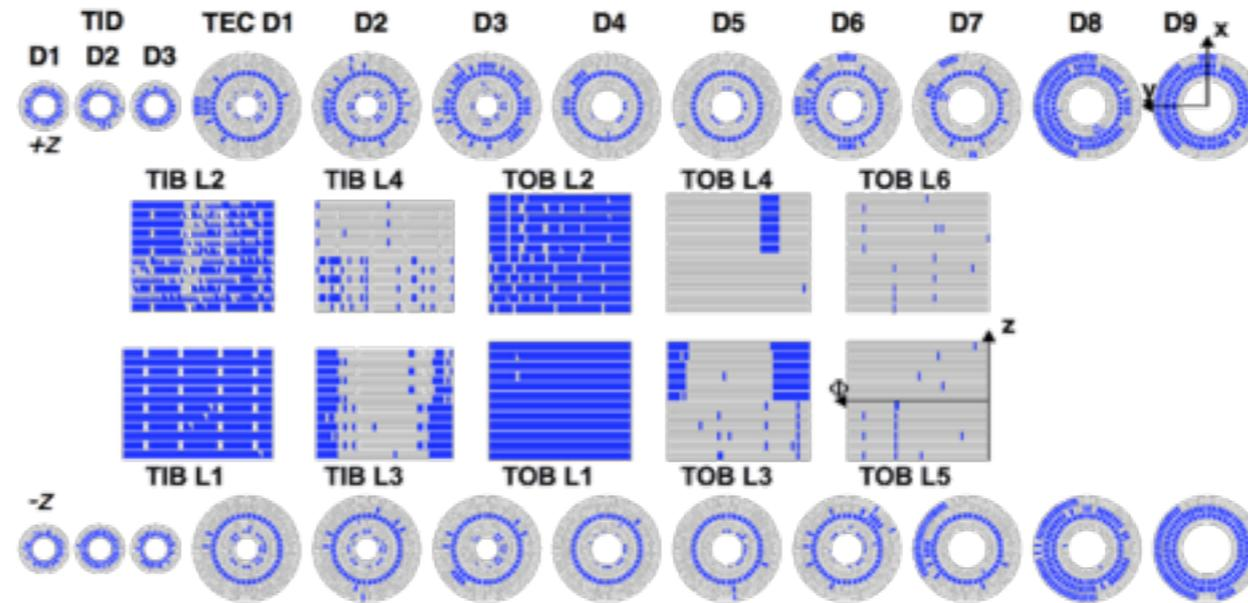
Blue tracker modules are inactive after  $1000 \text{ fb}^{-1}$  due to very high leakage currents induced by neutron fluence.
