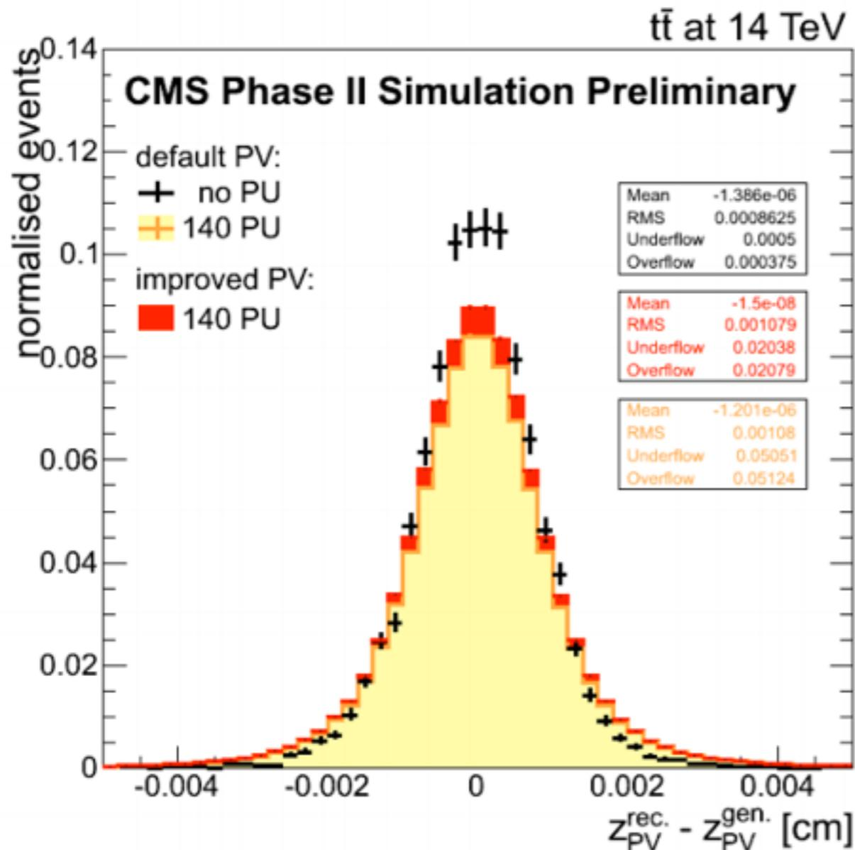
➔ 98% vertex finding efficiency with 140 PU
