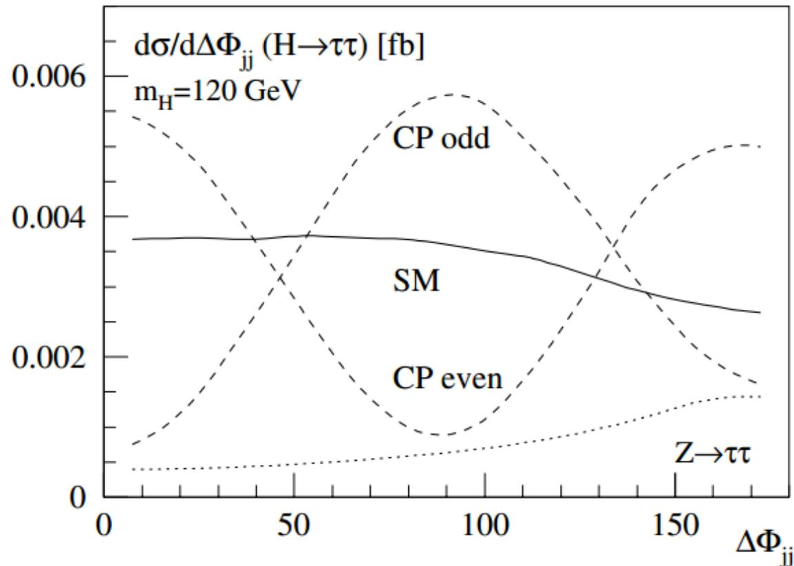
Azimuthal angular separation of tag jets in VBF
