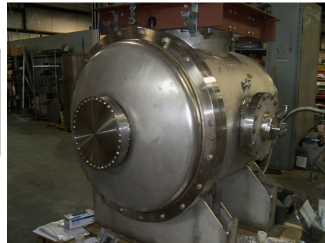
Modified ArgoNeuT Cryostat
