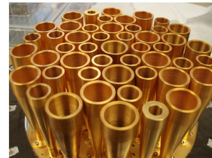
BICEP1: Feedhorns and NTD readout 150 and 100 GHz
