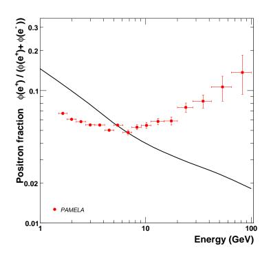
Satellite experiment;  $e^+e^-$  in cosmic rays Anomalous positron flux
