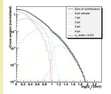
Differential 2  $\rightarrow$  3 jet rates at parton level by MadEvent + Pythia in  $p\bar{p} \rightarrow W$  + jets at the Tevatron,  $d_{\rm cut} = 10$  GeV (left),  $d_{\rm cut} = 30$  GeV (right).
