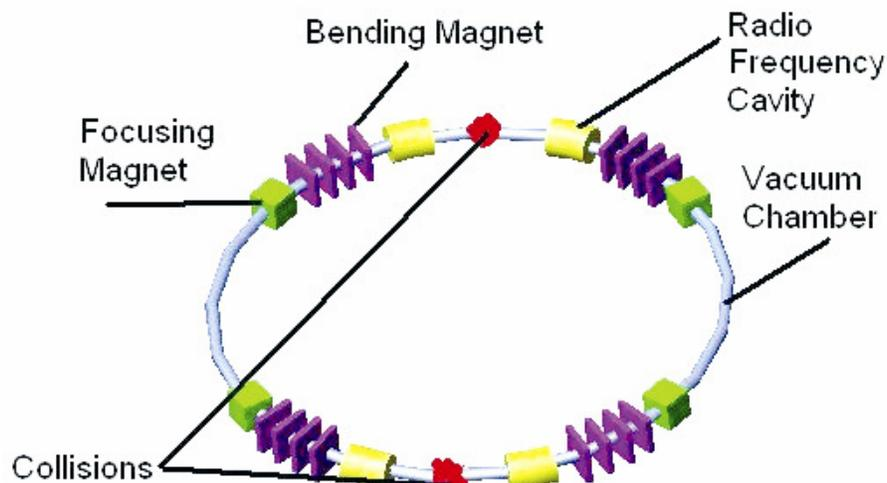
In an accelerator, focusing magnets and bending magnets guide the beam of particles around a ring. (Only a few of the bending magnets are shown here).
