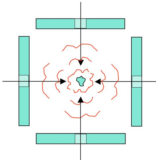
**Parallel tomographic coherent diffraction. N beams are directed through sample onto N detectors**
