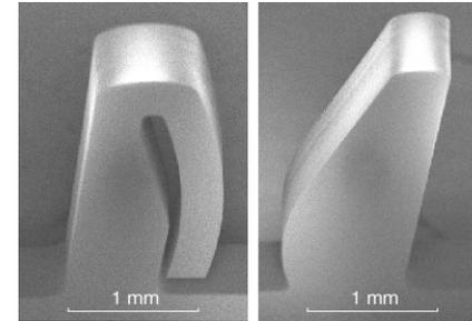
**Micromachined Si mirror nano-actuators for x-ray astronomy**
