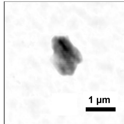
**Image of fish bone reconstructed solely from diffraction data**
