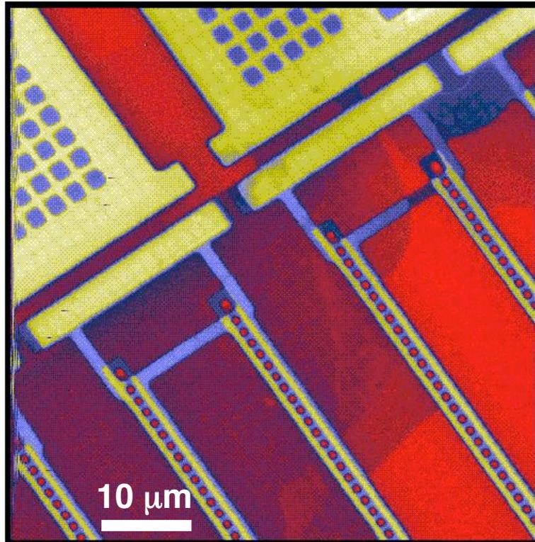
Scanning transmission x-ray micrograph (1830 eV) of a Cu/W/Si test device, showing interconnects and vias.
