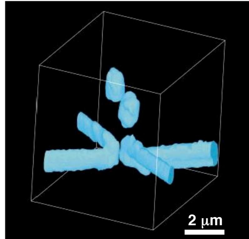
Bayesian reconstruction reconstruction of 13 STXM projections ( $\pm 69^\circ$ , 1573 eV) through two-level Al/W/Si test object. Al interconnects are joined by W vias. Two FIB markers are at top.
