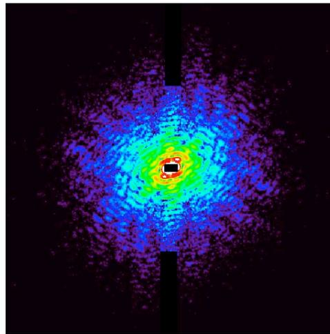
**Coherent diffraction pattern (2.2 keV) from a fish bone at a low mineralization state**
