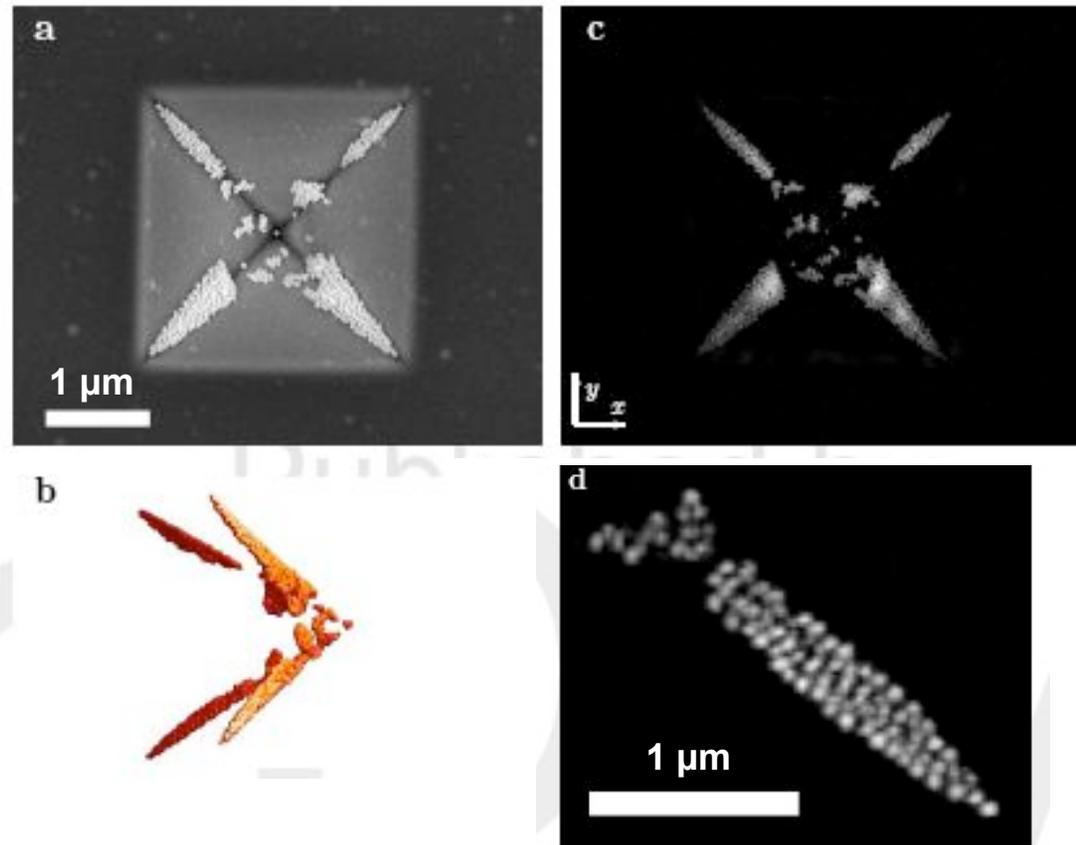
(a) SEM of pyramidal indentation in a 100-nm  $\text{Si}_3\text{N}_4$  membrane lined with 50-nm Au spheres. (b) 3D image reconstructed from 123 diffraction projections spanning  $-57^\circ$  to  $+66^\circ$ , using reality and positivity constraints. (c) Large DOF projection. (d) Enlarged region of (c).
