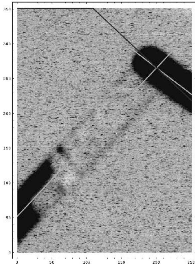
Normal-incidence scan of interconnect showing electromigration void detail.
