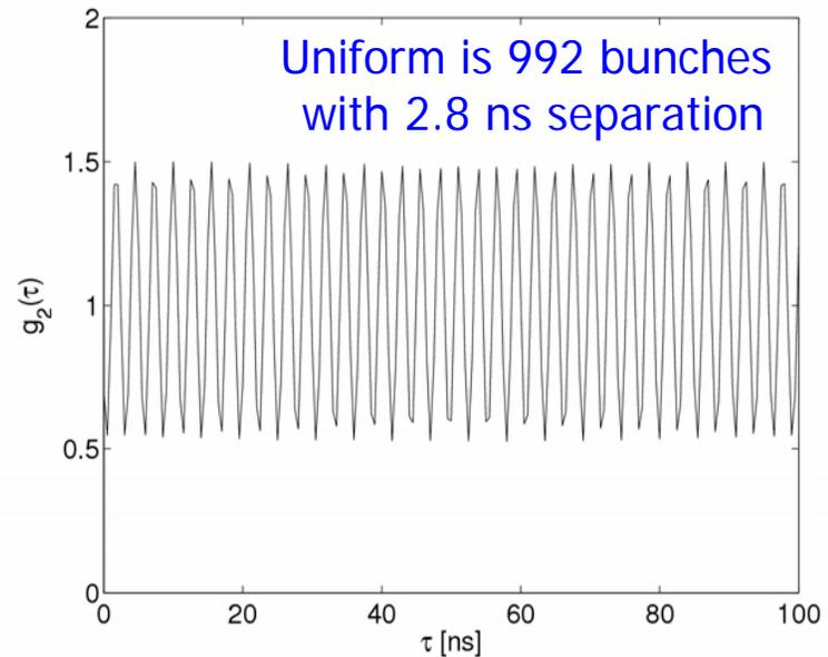
Data taken with APD detector and 2GHz scaler board
