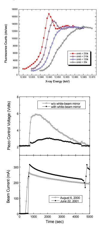
Figure 3. Energy scans around the Se Kedge at different bender settings 'cmrb' for the collimating mirror, upstream of the double crystal monochromator at F2 station. A higher numbers indicate a smaller bending radius. The shift in the edge position indicates a slight change in the deflection angle of the mirror when its bend is changed.
