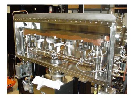
Figure 1. CHESS F-line white-beam mirror in its ultra-high-vacuum vessel. It consists of a flat Glidcop substrate with rhodium coating, a variable-force U-bender, and a system of springs for gravity compensation.
