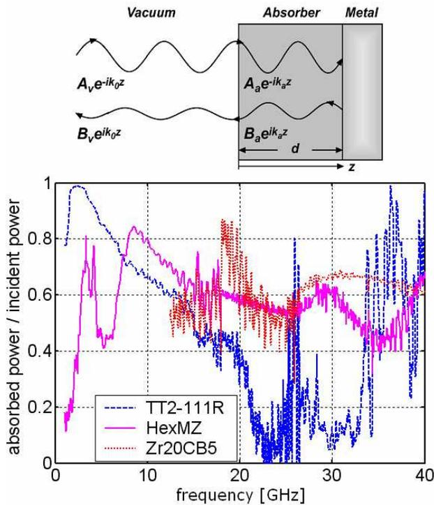
Fig. 7. Absorber model calculation ( $d = 3$  mm) based on measured  $\varepsilon$  and  $\mu$  at 80 K.
