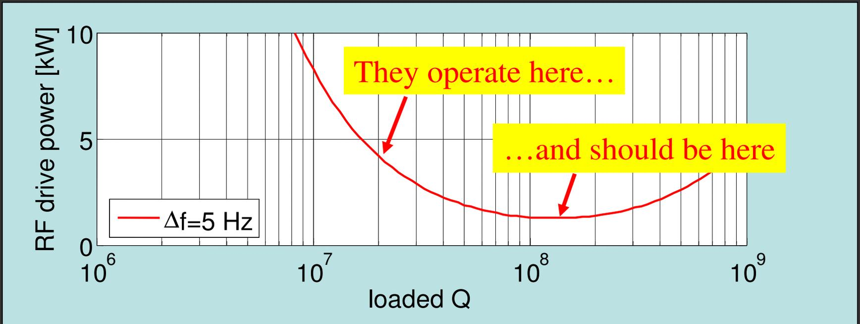
⇒ A good mechanical design results in very low microphonics levels, and would allow to run at a  $Q_L \approx 10^8$ !
