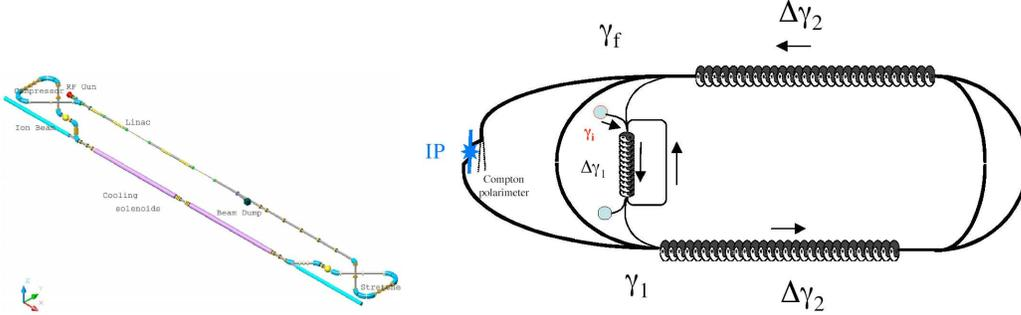
Fig. 4. Layout of an ERL for electron cooling of RHIC's ion beam and of the ERL that would provide electrons for collisions with the RHIC polarized proton and ion beams.
