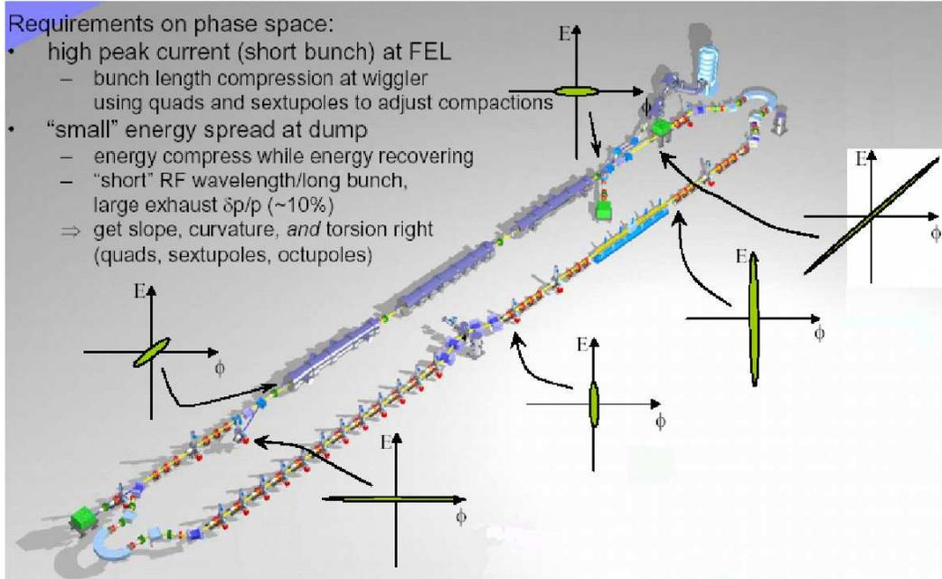
Fig. 6. Longitudinal phase-space manipulations in the JLAB FEL.
