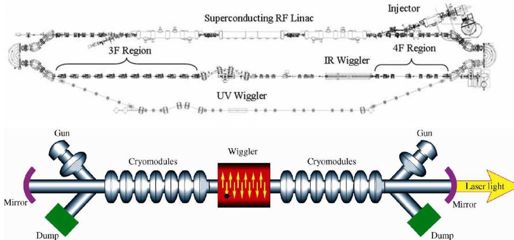
Fig. 2. Layout of the existing JLAB ERL-FEL and the proposed push-pull FEL.
