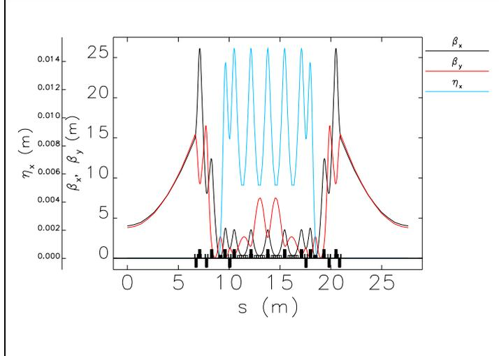
Fig. 5. Lattice functions for the XPS7 design.
