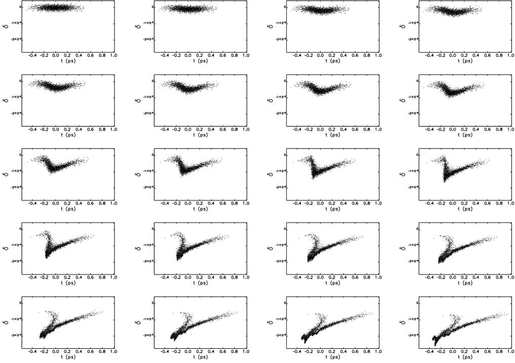
Fig. 8. Longitudinal phase space at the center of every other straight section in an APS lattice, assuming 100 pC, 50- $\mu\text{m}$  initial rms bunch length, 0.01% initial rms momentum spread, and 1- $\mu\text{m}$  initial normalized emittance [9].
