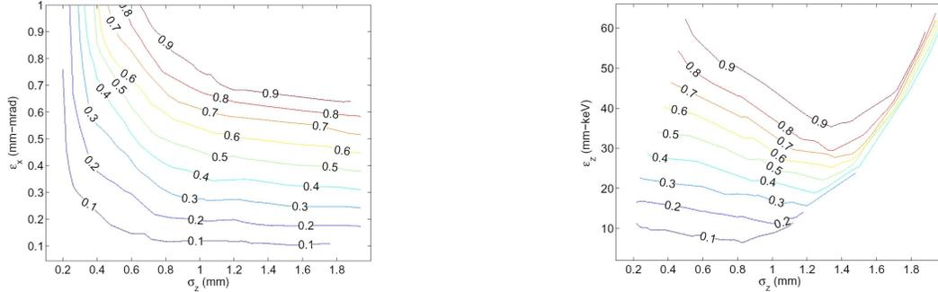
Fig. 1. Simulated small horizontal ( $\epsilon_x$ ) and longitudinal ( $\epsilon_z$ ) emittances from DC electron sources as a function of bunch length ( $\sigma_z$ ) and bunch charge in nC as indicated at each curve.
