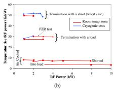
Figure 4: (a) Example of PT1000's temperature versus time. Measurements were made with HoBICAT cold and the waveguide shorted. (b) Summary of the all tests.
