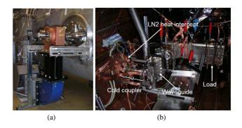
Figure 3: (a) Warm part of the coupler mounted on the outside of HoBiCAT. (b) Cold part of the coupler mounted in HoBiCAT along with the waveguide load. The copper straps are used to cool the 77-K and 2-K points of the coupler to about 100 K.
