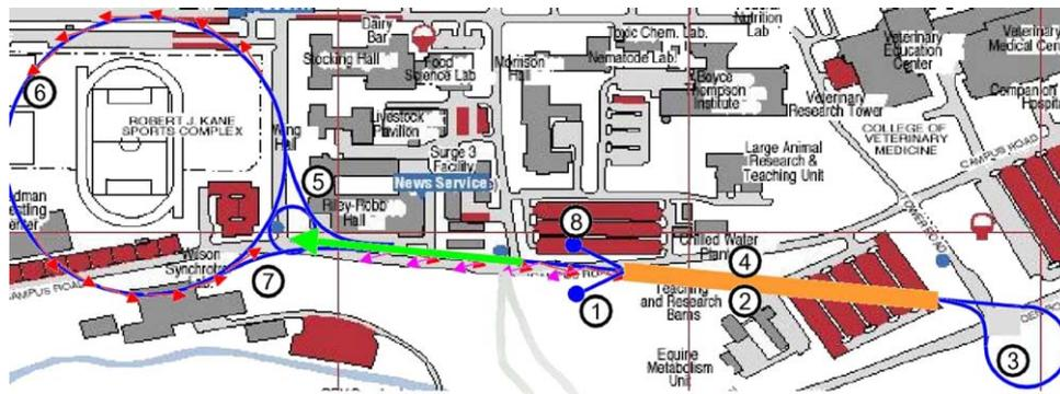
Fig. 1. An ERL in an extended CESR tunnel.
