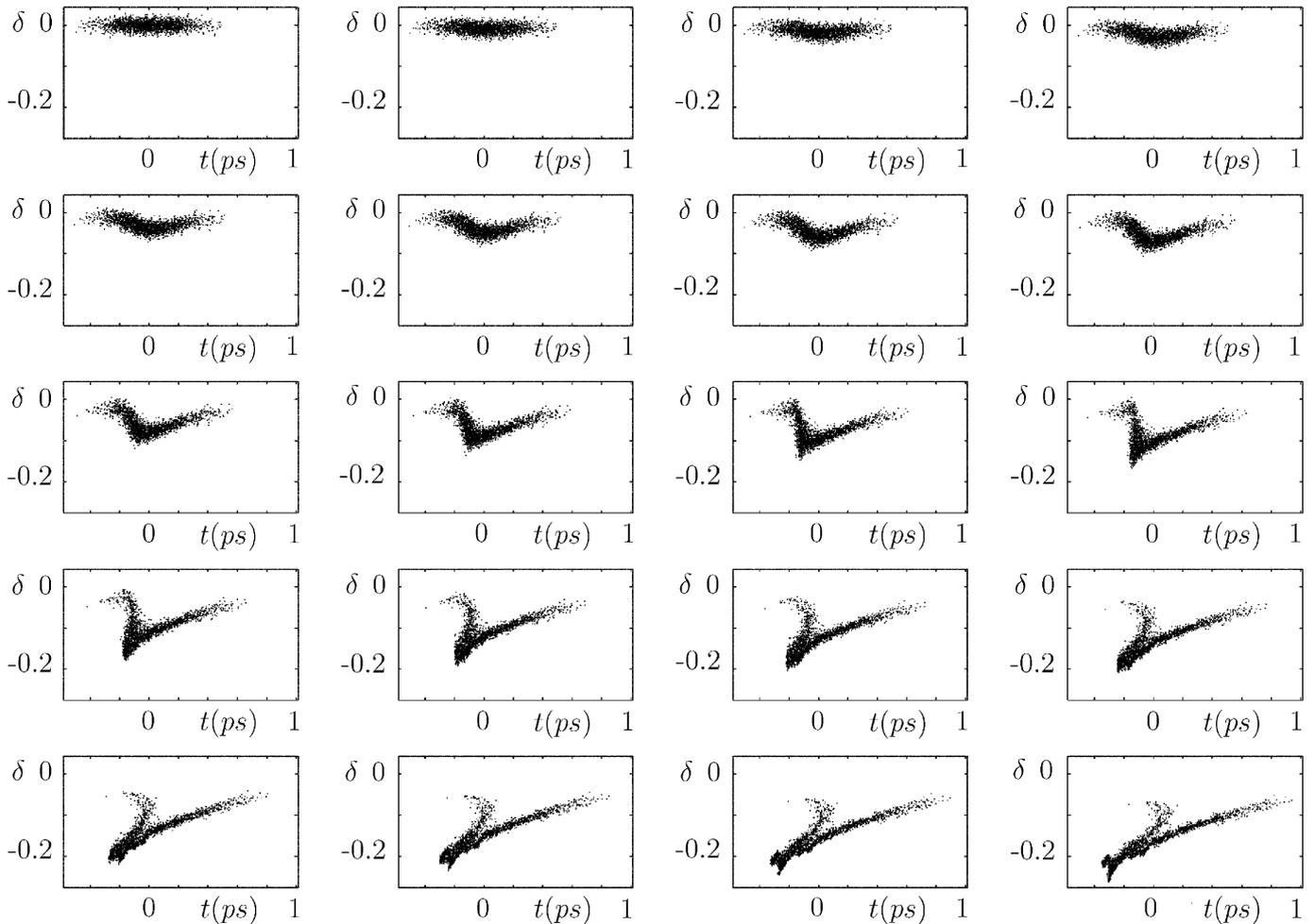
Fig. 8. Longitudinal phase space at the center of every other straight section in an APS lattice, assuming 100 pC, 50- $\mu$ m initial rms bunch length, 0.01% initial rms momentum spread, and 1- $\mu$ m initial normalized emittance [9].
