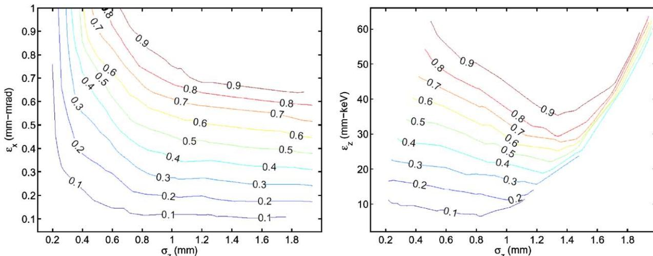
Fig. 1. Simulated small horizontal ( $\epsilon_x$ ) and longitudinal ( $\epsilon_z$ ) emittances from DC electron sources as a function of bunch length ( $\sigma_z$ ) and bunch charge in nC as indicated at each curve.
