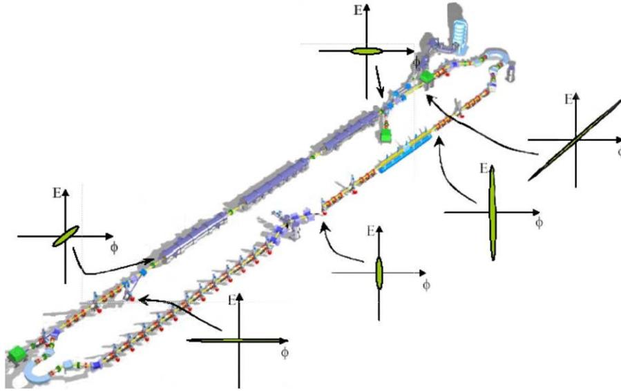
Fig. 6. Longitudinal phase-space manipulations in the JLAB FEL.
