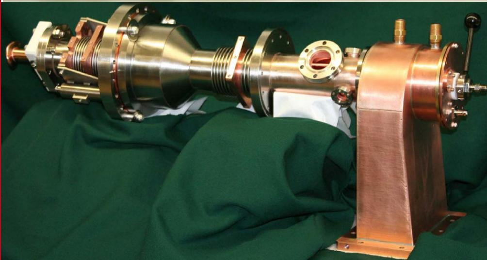
**Superconducting Cavities, high power input coupler, and high precision frequency tuners are all developed and build at Cornell (with outside collaborators)**
