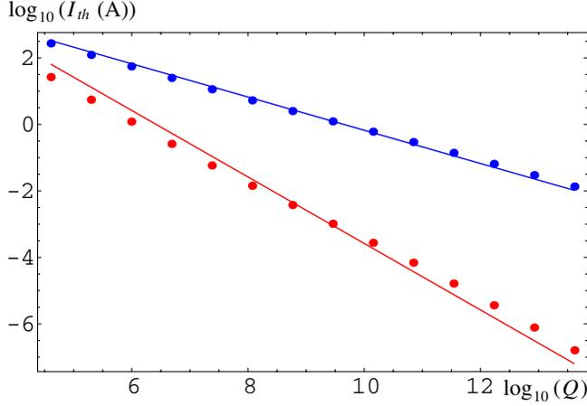
FIG. 1. (Color) The threshold with two modes in one cavity scales with  $Q^{-1}$  for a decoupled (red, bottom curve) and with  $Q^{-(1/2)}$  for a fully coupled optics (blue, top curve). The advantage of coupling thus diminishes for low  $Q$ .
