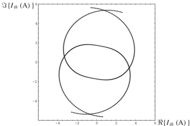
FIG. 3. Two eigenvalues trace out loops for  $I_0$  in the complex plane while  $\omega$  is varied.
