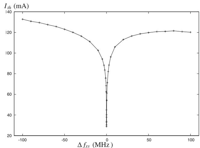
FIG. 7. Dependence of  $I_{th}$  on  $\Delta f_{xy}$  for the Cornell ERL.
