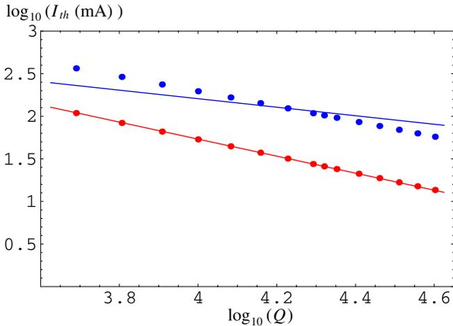
FIG. 2. (Color) Scaling with  $Q$  of the threshold increase due to coupling for the x-ray ERL upgrade of CESR. Red, bottom curve: scaling with  $Q^{-1}$  for a decoupled optics. Blue, top curve: a line indicates scaling with  $Q^{-(1/2)}$ , the points are obtained for a fully coupled optics.
