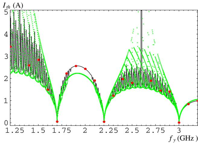
FIG. 5. (Color) Threshold current for one horizontal HOM with  $f_x = \omega_x/2\pi = 2.2$  GHz as a function of the frequency  $f_y$  of a vertical HOM. Black curve: dispersion relation; red dots: tracking; green dots: the approximation derived above. For clarity, a subinterval of this graph is shown in Fig. 6.
