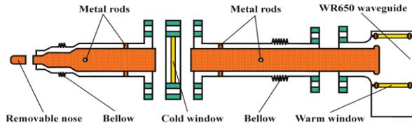
Figure 6: Conceptual drawing of the capacitive-coupling coupler.
