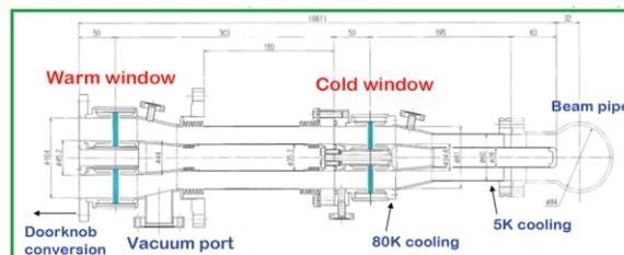
Figure 5: Drawing of the STF baseline cavity coupler.
