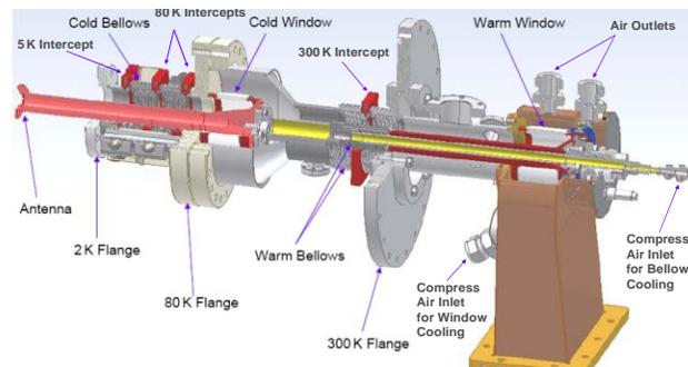
Figure 7: Cornell ERL injector input coupler.
