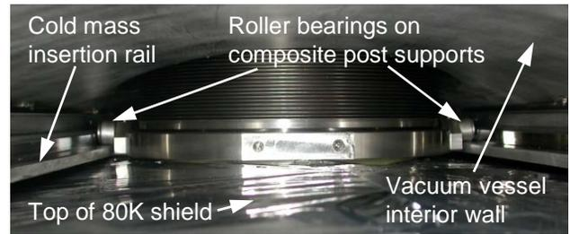
Figure 6: Cold mass insertion rails as seen from inside the vacuum vessel.
