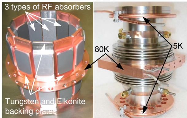
Figure 2: Cornell ERL Injector beamline HOM load.
