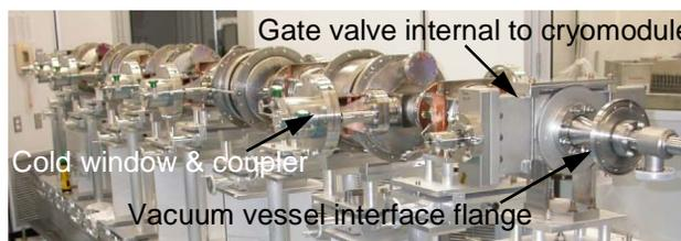
Figure 4: Completed beamline string in the clean room.
