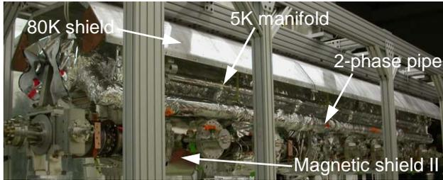
Figure 5: Cold mass assembly in a high-bay area.
