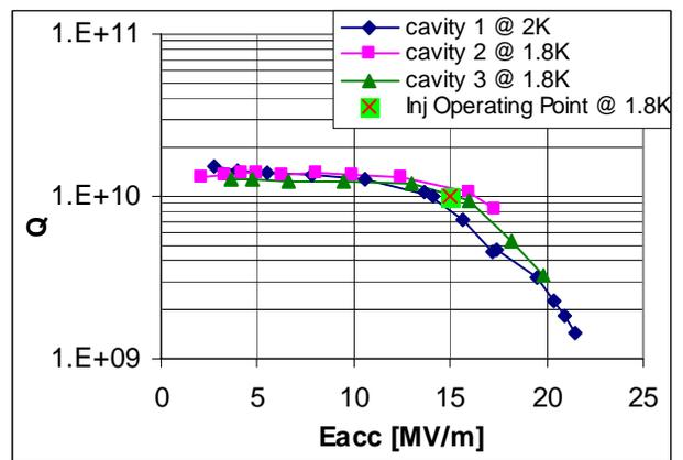
Figure 1: A sampling of  $Q_o$  vs.  $E$  curves from vertical tests for unbaked cavities.
