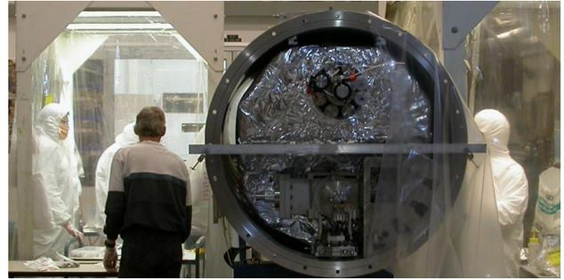
Figure 7: Portable clean rooms positioned on the sides of the vacuum vessel during warm coupler installation.
