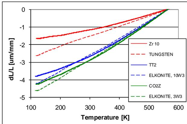
Figure 3: Thermal expansions of materials used in the beamline HOM loads.
