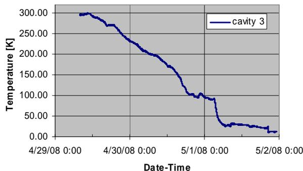
Figure 3: Temperature of cavity #3 during module cool-down.
