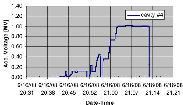
Figure 5: First ramp up of field in cavity #4.
