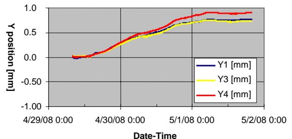
Figure 4: WPM data during cool-down of the injector module. (a) Horizontal position of WPM blocks on cavities 1, 3, 4, and 5. (b) Vertical position of WPM blocks on cavities 1, 3, and 4. WPM #2 is not functional.
