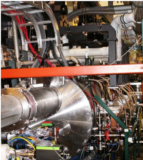
Figure 2: Injector cryomodule in the prototype ERL injector.
