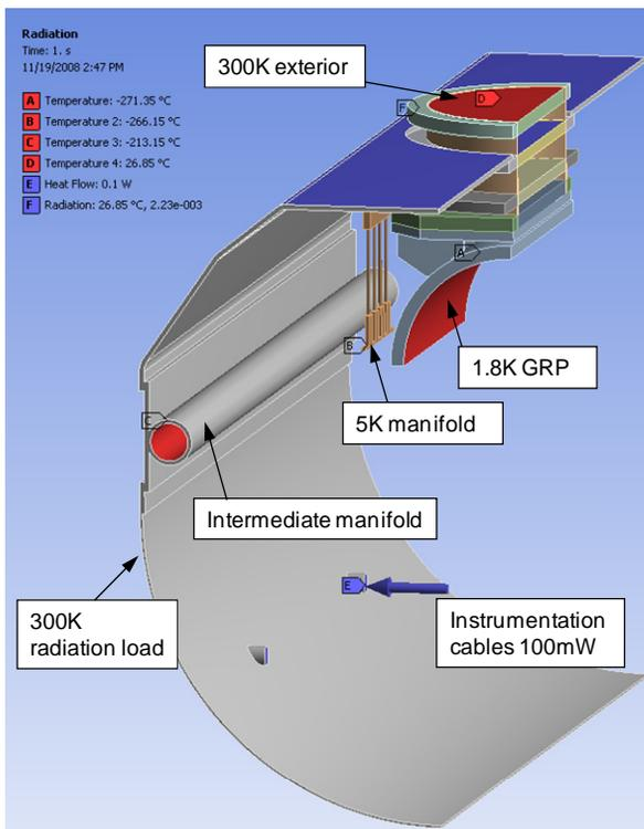
Figure 7: ANSYS model of  $1/8^{\text{th}}$  of the ERL linac module intermediate shield and composite support post.
