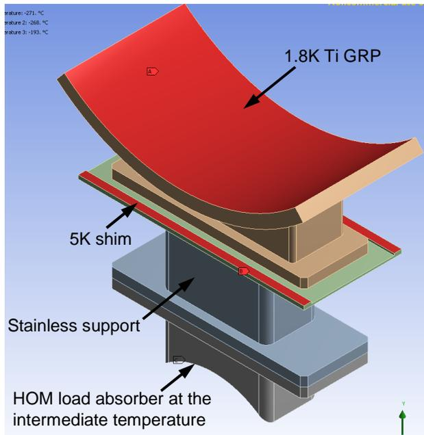
Figure 2: ANSYS model of the thermo-mechanical connection between the HOM body and the GRP.
