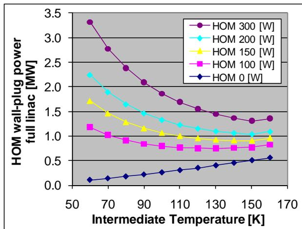
Figure 3: Linac wall-plug refrigeration power for the summed dynamic HOM absorber and static GRP support.
