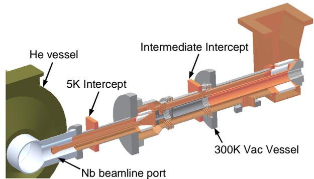
Figure 9: CAD model section view of the RF coupler attached to the SRF cavity.
