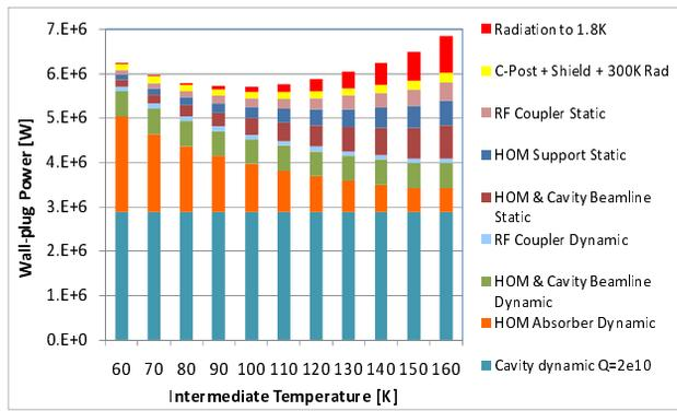
Figure 10: Wall-plug refrigeration power for a 64-module ERL linac as a function of the intermediate intercept temperature.
