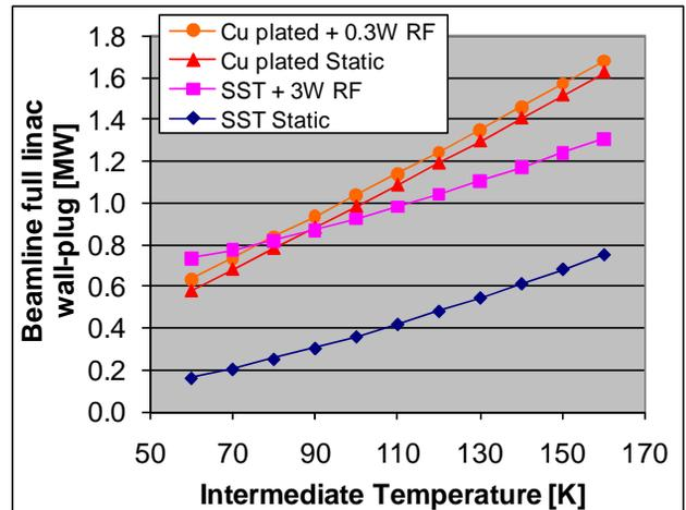
Figure 6: Wall-plug refrigeration power for the beamline between the cavity helium vessel and the HOM load absorber for the full linac.
