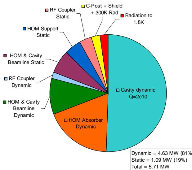
Figure 11: Distribution of wall-plug power loads for 64 cryomodules with a 100K intermediate temperature and cavity  $Q_0=2 \times 10^{10}$ .
