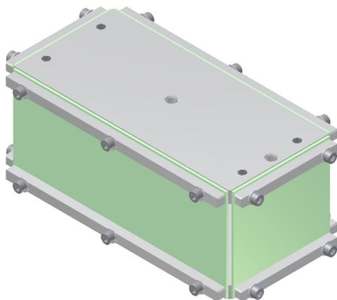
Figure 4: An alternate HOM support post comprised of 1/16" thick G-10 plates bolted to stainless steel plates.
