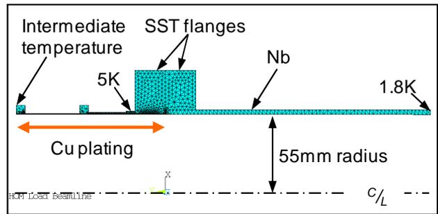
Figure 5: ANSYS 2D model of the axisymmetric beamline configuration between the cavity helium vessel and the HOM load absorber.
