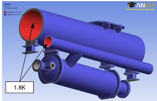
Figure 8: ANSYS model of  $1/7^{\text{th}}$  of the ERL linac module components nominally at 1.8K.
