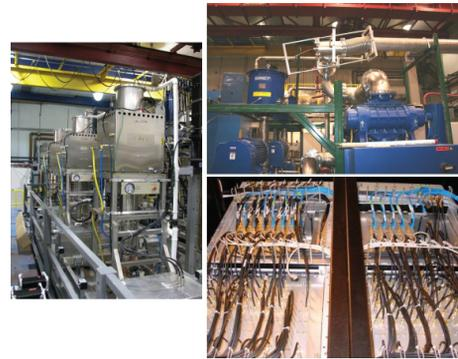
Figure 2: Left: 120 kW CW klystrons. Right, top: Cryogenic pumps. Right, bottom: LLRF control hardware.
