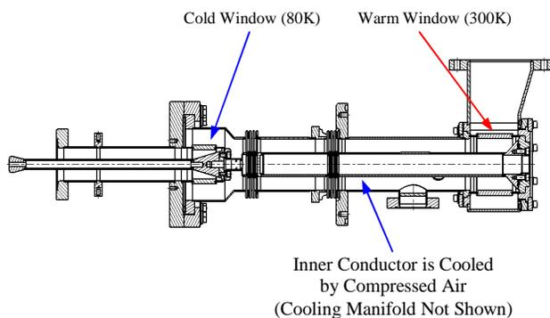
Figure 3: Section view of the coupler.
