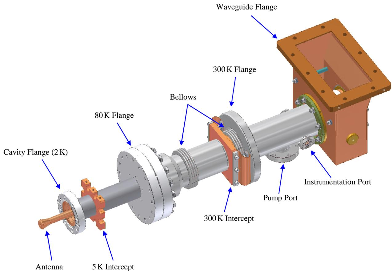
Figure 2: 3D CAD model of input coupler.
