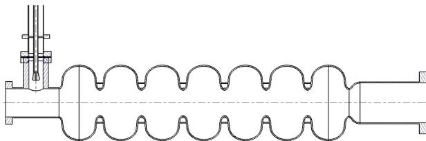
Figure 1: A 7-cell cavity with input coupler.
