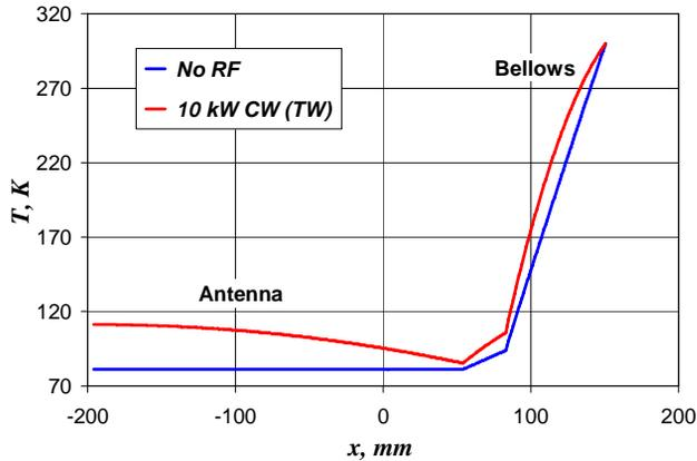
Figure 5: Temperature distribution along inner conductor.
