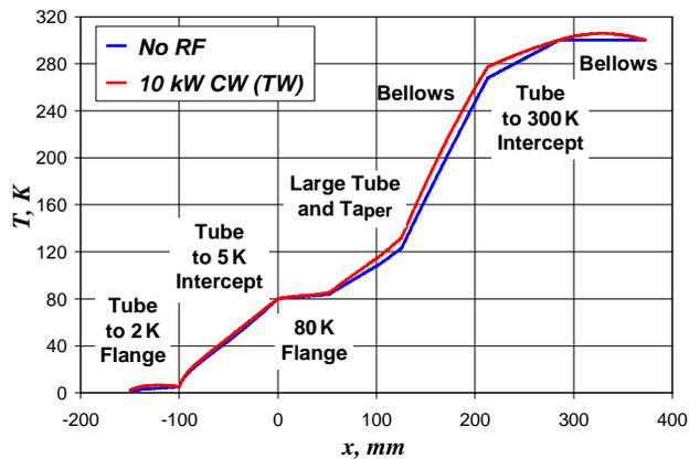
Figure 6: Temperature distribution along outer conductor.
