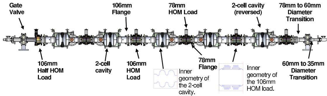
Figure 1: CAD model view of the Cornell ERL injector cryomodule beam line. Beam line components from left (beam entrance) to right (beam exit): gate valve; 106 mm half HOM load; first SRF cavity; 78 mm HOM load; second SRF cavity; 106 mm HOM load; third SRF cavity; 78 mm HOM load; fourth SRF cavity; 106 mm HOM load; fifth SRF cavity; 78 mm HOM load; 78 mm to 60 mm diameter transition; gate valve; 60 mm to 35 mm diameter transition.
