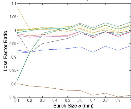
Figure 5: (color) Ratio of the loss factors calculated by ABCI and NOVO ( $k_{ABCI}/k_{NOVO}$ ). At shorter bunches, there is more discrepancy between the two programs. The legend is the same as in Figure 3 and 4.
