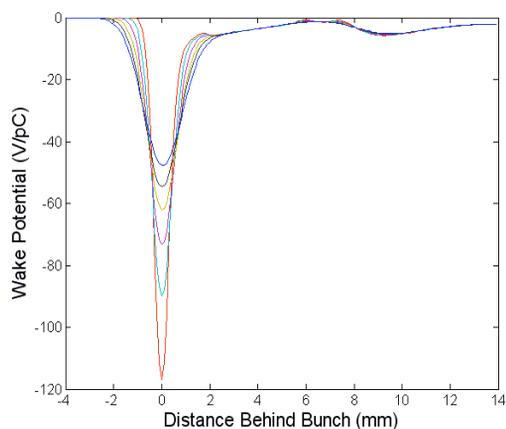
Figure 8: (color) Total wake potential the entire beam line of the injector cryomodule, as computed by adding individual wake potentials for each component, as computed by NOVO, for bunch sizes ranging from 0.1mm to 0.8mm.
