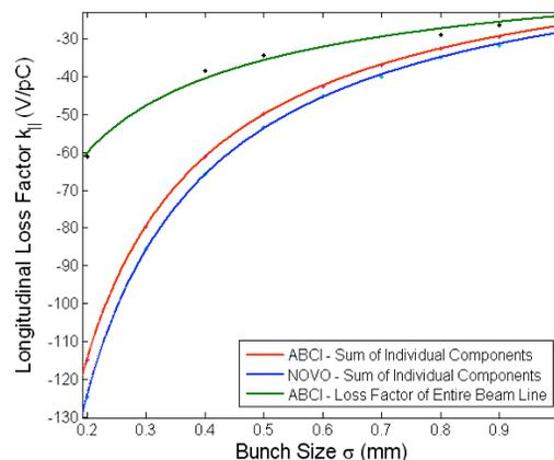
Figure 9: Total loss factor in the injector beamline as a function of bunch length. Notice that summing up the loss factors of the individual components overestimates the total loss factor, especially at short bunch lengths.
