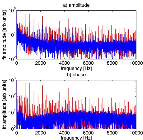
Figure 4: Field stability without (red) and with (blue) feed-forward klystron high-voltage ripple compensation. Top: FFT of the cavity field amplitude. Bottom: FFT of the cavity phase. The ripples in the HV are harmonics of 60 Hz.
