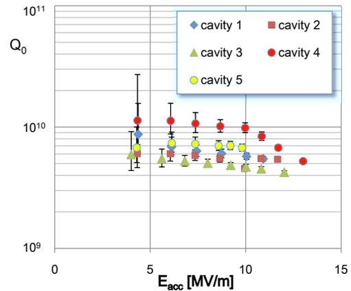
Figure 3: Intrinsic quality factor  $Q$  vs. accelerating field  $E_{acc}$  of the injector SRF cavities at 1.8K after rework of the cryomodule.
