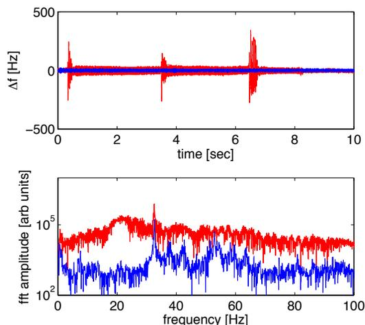
Figure 6: Cavity detuning before (red) and after (blue) setting up LHe flow through the warm-up cool-down pipe. Top: Detuning vs. time. Bottom: Microphonics spectrum.
