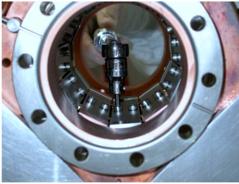
Figure 2: Reassembly of an ERL injector beamline HOM load in a clean room after panel EDM cuts and thorough cleaning. The remaining RF absorber tiles face outwards, and the fields by potential charging of the tiles are shielded from the beam by the metallic substrate.
