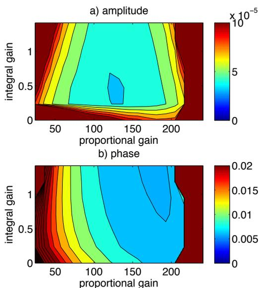
Figure 5: Integral and proportional gain scan to optimize the gains used in the field control loop. Top: Relative amplitude stability (blue:  $\sigma_A/A < 4 \times 10^{-5}$ ). Bottom: Phase stability (blue:  $\sigma_p < 0.01^\circ$ ).
