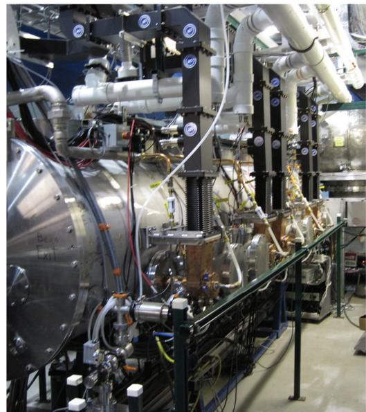
Figure 4: Superconducting booster module of the Cornell ERL injector, capable of providing beam powers of up to 500 kW via five two-cell cavities.
