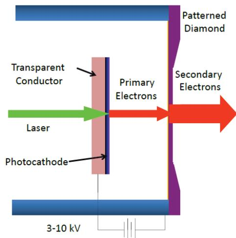
Figure 10: Principle of the diamond amplifier (from [18]).
