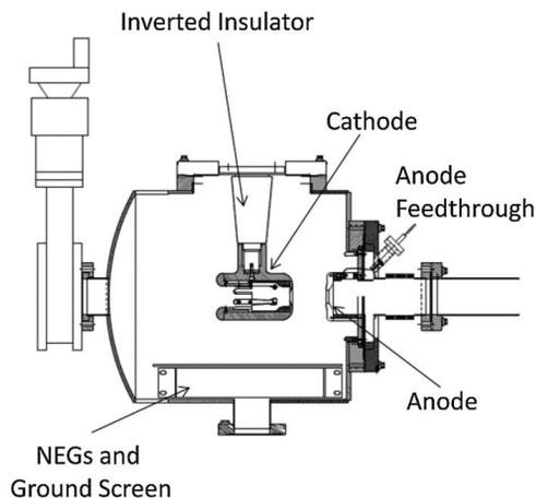
Figure 3: Schematic of an “inverted” DC gun (from [6]).
