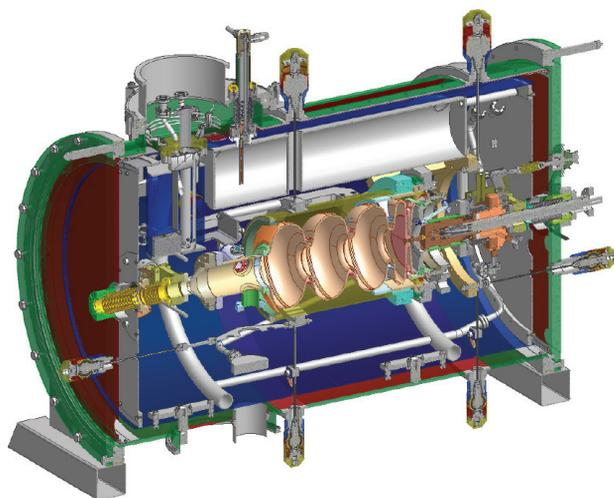
Figure 8: Schematic of the superconducting ELBE photoinjector (from [15]).
