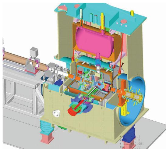
Figure 9: High-current superconducting gun developed at BNL (from [16]).
