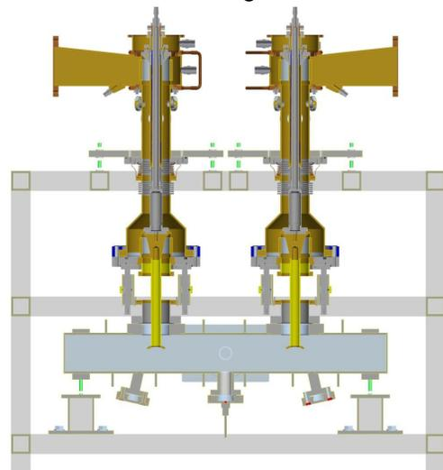
Figure 1: Coupler Test Stand
