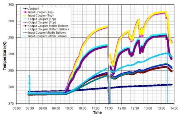
Figure 4: Thermocouple Temperatures for CW Conditioning Run.
