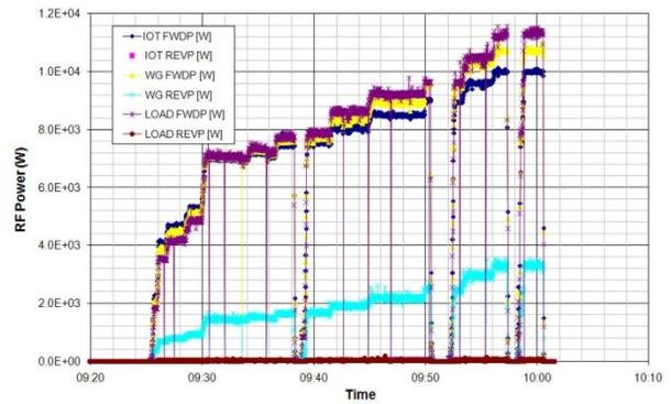
Figure 5: RF Power Levels for Pulsed Conditioning Run.
