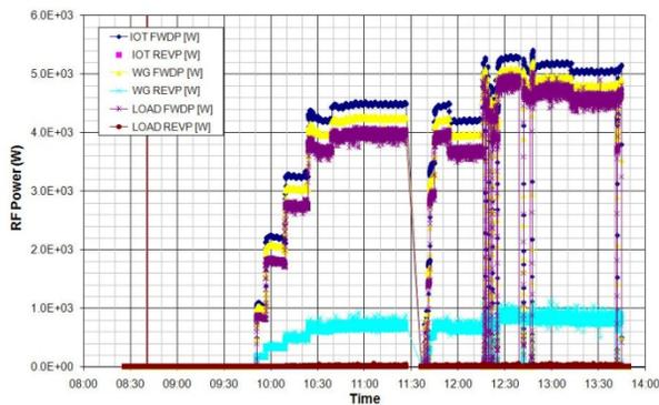
Figure 3: RF Power Levels for CW Conditioning Run.
