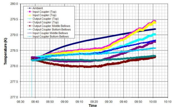
Figure 6: Thermocouple Temperatures for Pulsed Conditioning Run.
