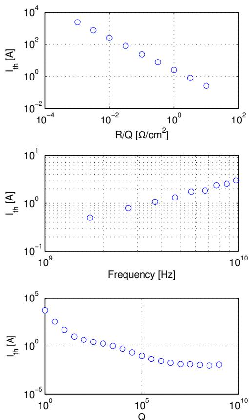
Figure 1: Scaling of the threshold current vs  $R/Q$ , frequency and  $Q$ , assuming a frequency spread  $\sigma_f/f = 5 \times 10^{-3}$ . For all plots,  $R/Q = 5 \Omega/\text{cm}^2$ ,  $Q = 10^4$ ,  $f = 1.7$  GHz, except when a given parameter is the independent variable. The circles mark the threshold current obtained by at least 90% of the random runs.
