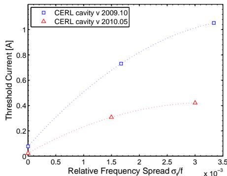
Figure 4: Beam break-up current versus relative frequency spread for simulated ERLs. Blue points are the old cavity design with an IFIA, and red marks the new cavity design with a realistic CNT absorber. The new design only supports half the current of the old design, but its absorber properties are more realistic than those of the old design. To achieve 100 mA threshold current with the new design, a relative frequency spread of  $3.3 \times 10^{-4}$  is required.
