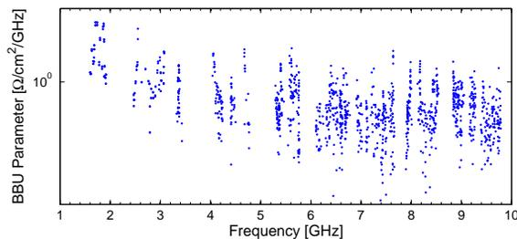
Figure 3: Beam break-up parameter vs Frequency for 1692 dipole HOMs for the optimized 7-cell cavity.
