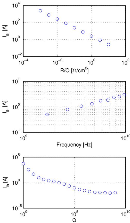
Figure 1: Scaling of the threshold current vs  $R/Q$ , frequency and  $Q$ , assuming a frequency spread  $\sigma_f/f = 5 \times 10^{-3}$ . For all plots,  $R/Q = 5 \Omega/\text{cm}^2$ ,  $Q = 10^4$ ,  $f = 1.7$  GHz, except when a given parameter is the independent variable. The circles mark the threshold current obtained by at least 90% of the random runs.
