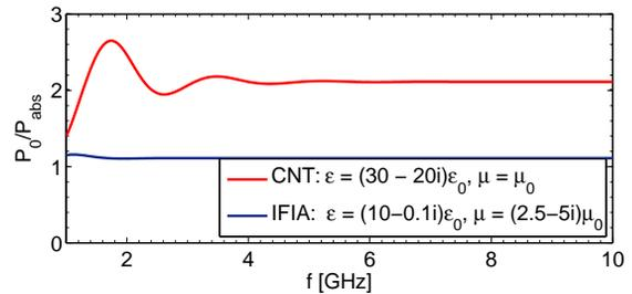
Figure 5: Total HOM power,  $P_0$ , over power dissipated in absorber,  $P_{abs}$ , vs HOM frequency assuming a plane wave incident normally on an ideal 3 cm thick absorber.
