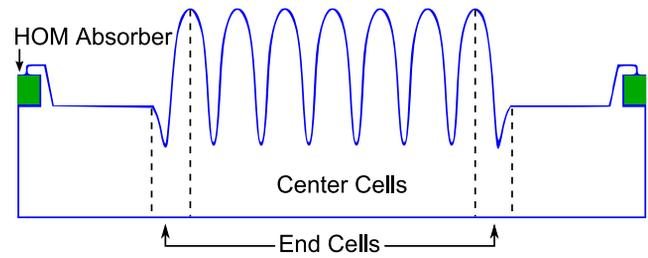
Figure 2: Schematic of 7-cell. The end cell designs are optimized to maximize  $I_{th}$ . HOM absorbers appear in green.
