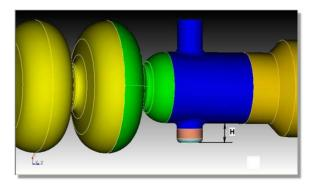
Figure 2: Coupler region of 7-cell cavity geometry. Orange cylinder illustrates method used to tune the compensation stub height, by an additional amount H.
