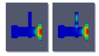
Figure 1: Coupler region of cavity showing fields for two frequencies. Left is on resonance for the 1.3 GHz 7-cell structure and right is obtained by launching a wave through the fundamental power coupler with a frequency 14 kHz higher.
