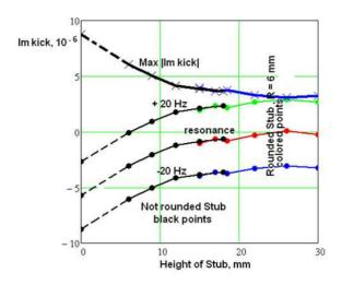
Figure 6: Imaginary part of the normalized coupler kick as a function of compensation stub height. The imaginary component of  $\kappa$  contributes to emittance growth. A stub height of zero corresponds to no compensation stub.
