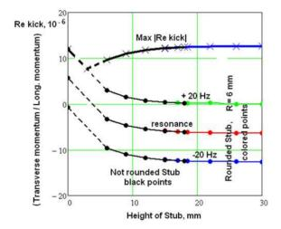
Figure 5: Real part of the normalized coupler kick as a function of compensation stub height. The real part of  $\kappa$  contributes to the transverse kick of the beam. A stub height of zero corresponds to no compensation stub. The  $\pm 20~{\rm Hz}$  values correspond to expected detuning due to microphonics for an operational 7-cell main linac cavity. Top blue line is the worst value of the coupler kick within  $\pm 20~{\rm Hz}$  of the resonant frequency.
