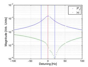
Figure 4: Magnitude of the longitudinal momentum gain and normalized coupler kick versus frequency. The blue lines mark  $\pm 20$  Hz, which is typical detuning operation for the ERL.
