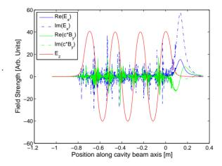
Figure 3: Real and imaginary parts of the field components along the beam axis of the 7-cell cavity. The longitudinal electric field has been scaled down by a factor of 500 for clarity. Note that  $c \cdot B$  is plotted so that the magnetic field effect can be directly compared with the effect of the electric field. The coupler is located at approximately z=0.14 m, where a small oscillation shows the field interaction with the bunch.
