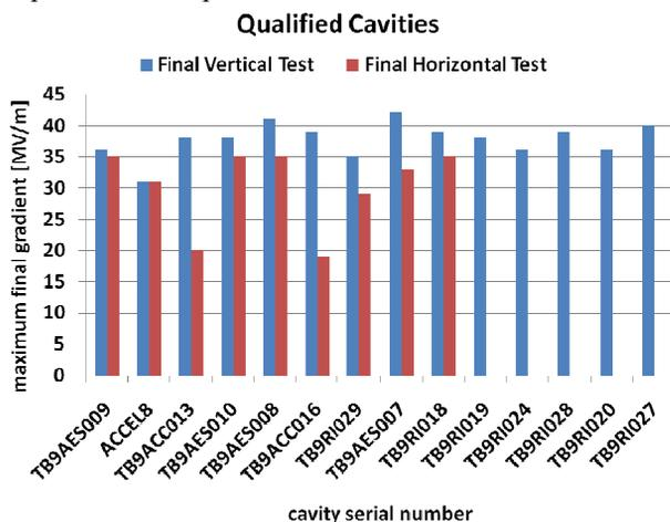
Figure 3: Comparison of final results from bare (blue) and dressed (red) cavity tests, ordered by horizontal test date.
