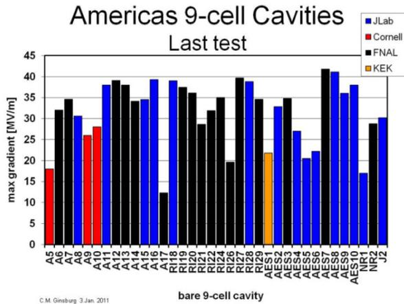
Figure 1: Bare cavity gradient performance in the most recent qualification test as of Jan.3,2011. Tests performed at FNAL are shown by the black bars. Surface processing location is typically, but not solely, the test lab shown.
