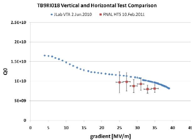
Figure 2: An example  $Q_0$  as a function of  $E_{acc}$ , showing both bare cavity (blue) and dressed cavity performance. The bare cavity test data are courtesy of JLab.
