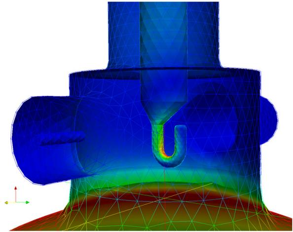
Figure 4: Magnetic field distribution near an off-center hook coupler tip calculated by Omega3P.
