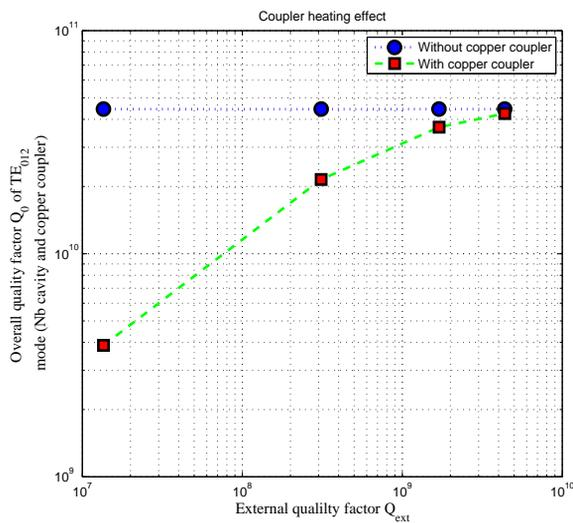
Figure 6: Host cavity  $Q_0$  degradation due to coupler penetration.
