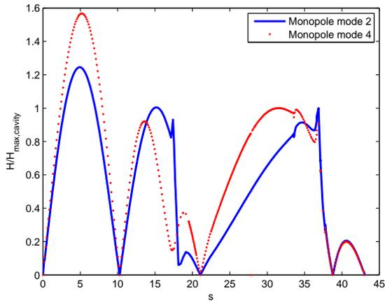
Figure 2: Normalized surface magnetic field along the sample plate and walls of the host cavity. Sample plate:  $s=0$  to 10 cm. Host cavity:  $s=10$  to 43 cm. mode 2:  $TE_{012}$ , mode 4:  $TE_{013}$
