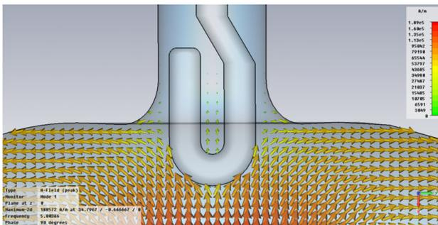
Figure 3: Magnetic field distribution near a "Saclay" style loop coupler tip calculated by MWS
