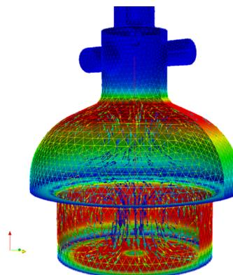
(a) Spatial magnetic field distribution of  $TE_{012}$  mode, red indicates high magnetic field, the maximum magnetic field on the sample plate is 1.24 times higher than on host cavity wall
