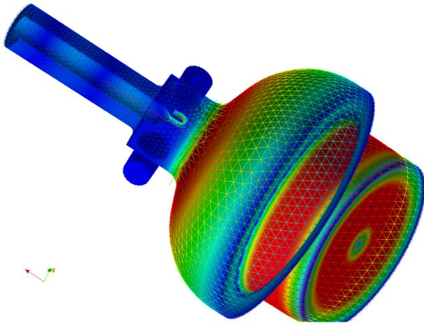
Figure 7:  $TE_{012}$  magnetic field distribution of TE mushroom cavity with full length input coupler port calculated by Omega3P.
