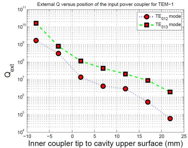
Figure 5:  $Q_{ext}$  dependence on coupler penetration depth into cavity.
