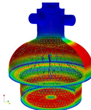
(b) Spatial magnetic field distribution of  $TE_{013}$  mode, red indicates high magnetic field, the maximum magnetic field on the sample plate is 1.57 times higher than on host cavity wall
