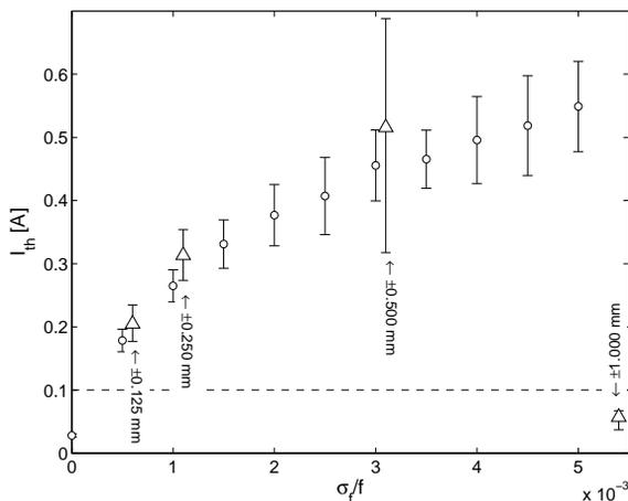
Figure 6: Threshold current versus frequency spread (which is related to fabrication variation size). Circles mark points obtained from the HOM spectrum of the optimized cavity with artificially introduced frequency spread, and triangles denote the mean values from realistic ERLs with cavity shape errors and no artificial frequency spread. The error bars mark the lowest and highest current obtained by the middle 80% of the runs.
