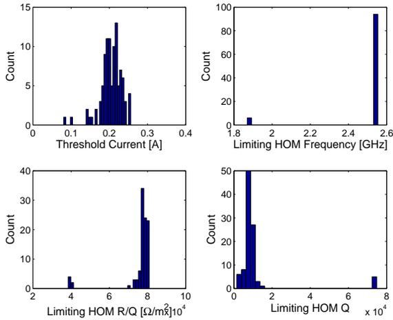
Figure 1: Histogram of BBU results for  $\pm 0.125$  mm error. Top left shows the histogram of threshold current. Other histograms show the frequency,  $R/Q$  and  $Q_L$  of the mode causing beam break-up.
