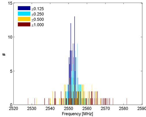
Figure 5: Histogram of frequency distribution of modes from the 2.5 GHz band, for the four error sizes. As the error size increases the RMS frequency spread of the modes also increases.
