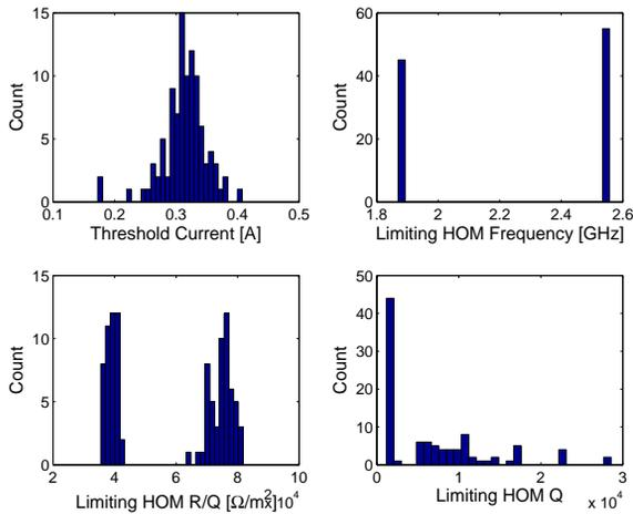
Figure 2: Histogram of BBU results for  $\pm 0.250$  mm error. Top left shows the histogram of threshold current. Other histograms show the frequency,  $R/Q$  and  $Q_L$  of the mode causing beam break-up.
