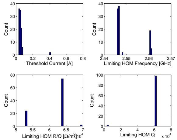
Figure 4: Histogram of BBU results for  $\pm 1.000$  mm error. Top left shows the histogram of threshold current. Other histograms show the frequency,  $R/Q$  and  $Q_L$  of the mode causing beam break-up.
