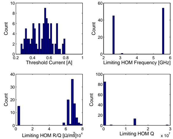
Figure 3: Histogram of BBU results for  $\pm 0.500$  mm error. Top left shows the histogram of threshold current. Other histograms show the frequency,  $R/Q$  and  $Q_L$  of the mode causing beam break-up.
