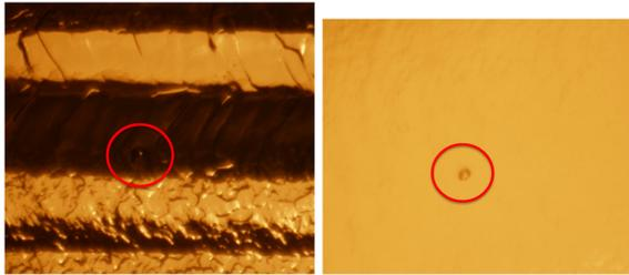
Figure 8: Defects observed in NR1-2 not causing quench below 27 MV/m.
