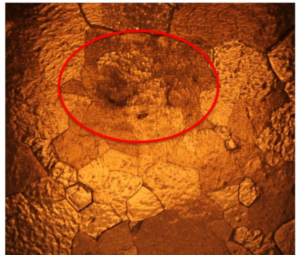
Figure 11: Discolored area observed on LR1-3. It did not cause quench.
