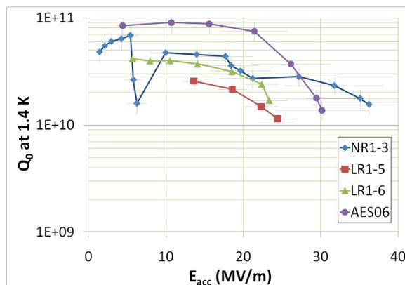
Figure 1: Q vs E curves of cavities tested at 1.4 K.
