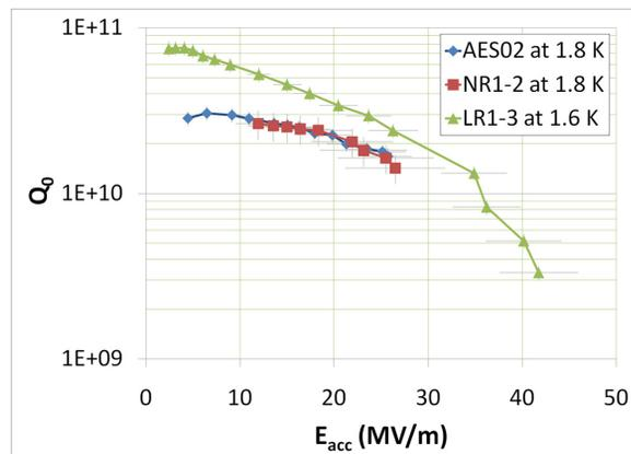
Figure 2: Q vs E curves of cavities tested at 1.6 and 1.8 K.
