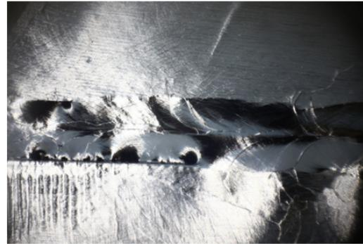
Figure 15: A typical area on the surface of LR1-6. Like the quench spot, it shows large, sharp topological features.
