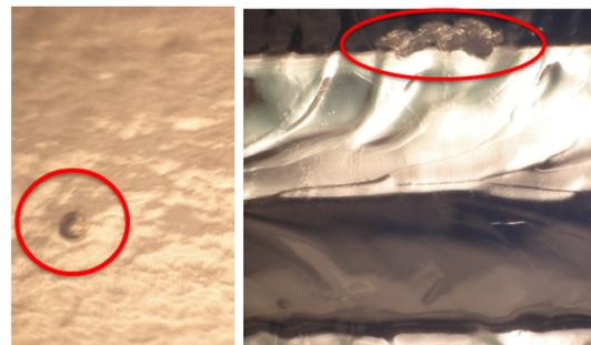
Figure 6: Defects observed in AES06 not causing quench below 30 MV/m.
