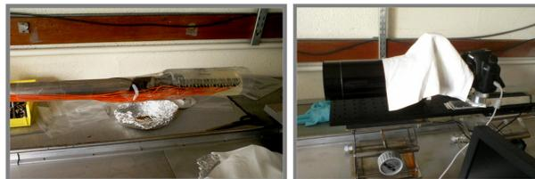
Figure 3: Optical inspection system light and mirror (left) and camera and telescope (right).
