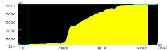
Figure 13: Confocal microscope rendering (above) and profile (below) of 500 um high step in surface mold of quench spot.
