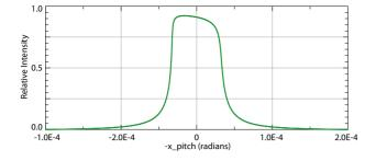
Figure 1: Rocking curves for a Si111 symmetric Bragg Crystal for 10 KeV photons. The curves were produced by varying the x\_pitch attribute of the crystal. The Darwin curves are centered on x\_pitch = 0 since Bmad adjusts the reference trajectory to go through the "Q" point at the center of the dispersion surface.
