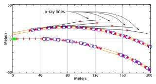
Figure 2: Simple example of the Cornell ERL with four xray lines. The x-ray lines are composed of two drift spaces represented by a line with a mirror element, represented by a circle, in between.
