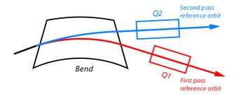
Figure 3: At the beginning or end of a multipass section the reference orbits on the different passes will diverge. The bookkeeper details of this are handled by Bmad. Shown is a bend at the end of a multipass section.
