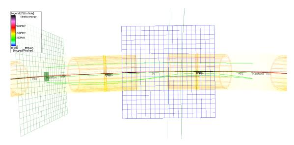
Figure 3.1.3: Matched orbits (green) for the four CBETA energies through an FFAG arc cell made with OPERA-3D field maps generated from Halbach magnets. The orange cylinders represent the approximate apertures of the vacuum pipe and the grids are 1 cm per square.
