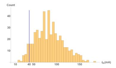
Figure 2.16.2: 500 BBU simulation results of  $I_{\rm th}$  for the CBETA 4-pass lattice. Each cavity is assigned with a random set of 10 dipole HOMs ( $\epsilon=125\,\mu{\rm m}$ ). The blue line indicates the UPP of 40mA for 4-pass machine.
