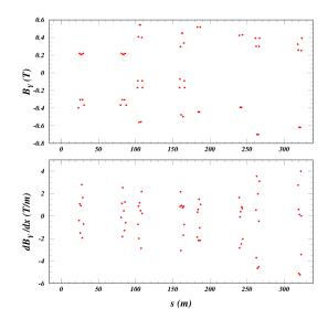
Figure 2.5.3: Distributions of required splitter dipole and quadrupole magnet field strengths versus the longitudinal orbit coordinate s. The magnets are thus ordered from left to right S1-R1-S2-R2-S3-R3-S4-R4.
