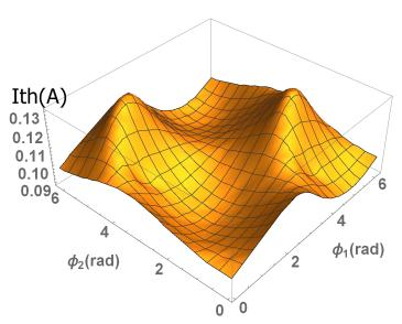
Figure 2.16.7: A scan of BBU  $I_{\rm th}$  over the two free phases for the CBETA 4-pass lattice with x-y coupling. Each cavity is assigned with a random set of 3 dipole HOMs in both x and y polarization. ( $\epsilon=125\,\mu{\rm m}$ ). For this particular HOM assignment,  $I_{\rm th}$  ranges from 89mA to 131mA.
