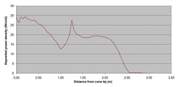
Figure 4.6.3: Energy deposition for 600 kW beam power at optimized condition
