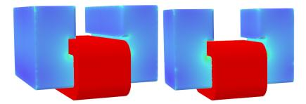
Figure 2.5.8: Color contours of the modeled field magnitude on the steel surface of the vertical corrector magnet models for a central field value of 160 G. The field ranges from 12 G (blue) to 400 G (green) in the visible region. Under the coil the field reaches 700 G. Left: 10-cm-long model with field integral 0.022 T-m. Right: 5-cm-long model with field integral 0.015 T-m.
