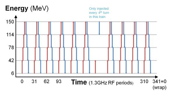
Figure 2.8.1: Bunch pattern produced in the eRHIC-like mode that has a circumference of  $h=343~\mathrm{RF}$  wavelengths but a time periodicity of 341 RF periods.
