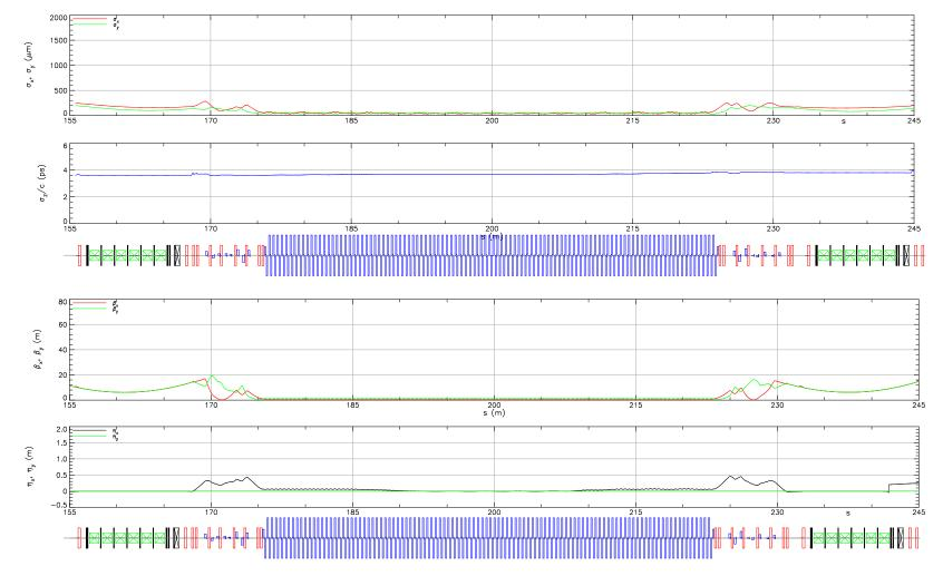
Figure 2.15.5: Optics and beam sizes for pass 3, 114 MeV
