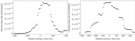
(a) Gamma dose rate outside shielding wall in (b) Neutron dose rate outside shielding wall in LOE.  $\,$
