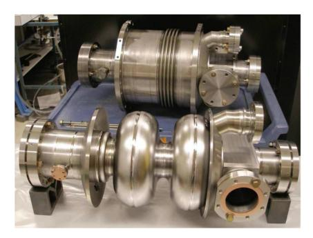
Figure 4.5.4: 2-cell cavity before and after welding the helium vessel
