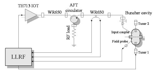
Figure 4.4.2: Block diagram of the buncher cavity RF system.
