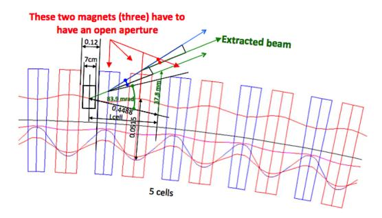
Figure 2.7.1: Orbit of the extracted beam through couple of FFAG arc magnets.
