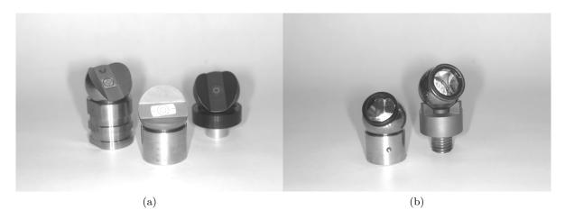
Figure 11.1.1: Left: Sphere mounted the odolite target. Right: Sphere mounted glass and air reflectors.
