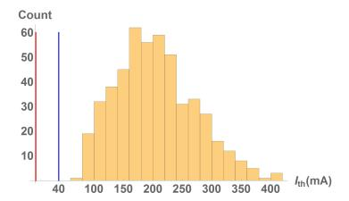
Figure 2.16.1: 500 BBU simulation results of  $I_{\rm th}$  for the CBETA 1-pass lattice. Each cavity is assigned with a random set of 10 dipole HOMs ( $\epsilon=125\,\mu{\rm m}$ ). The red line indicates the KPP of 1mA, while the blue line indicates the UPP 40mA for 1-pass machine.
