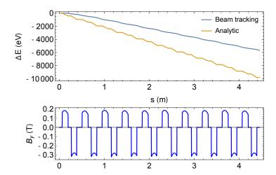
Figure 2.9.1: CSR average energy losses through 10 FFAG cells for a bunch at energy 42 MeV, 77 pC charge, and 3 ps duration by tracking in Bmad. The analytic calculation is simply accumulating  $0.35 \times W_0$  with curvature based on the local magnetic field  $B_y$ , and represents a lower limit on the average loss.
