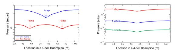
Figure 7.4.1: a) Simulated pressure profiles in a 4-cell FFAG beam pipe, comparing one-pump and two-pump per beam pipe configurations and b) Simulated vacuum improvement with time for a 4-cell FFAG beam pipe in one-pump configuration.
