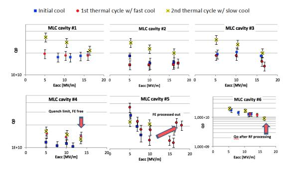
Figure 5.5.5: Summary of the MLC cavity performance. All data were taken at 1.8 K. Two cavities had to be RF processed to increase the field and to remove field emission. Cavity #4 is still limited by an early quench, but administrative procedures (for now) prevented us from processing this cavity further.
