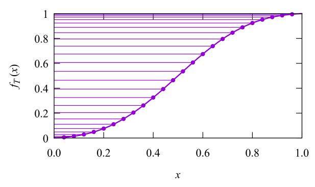
Figure 2.6.7:  $f_T(x)$  used for the transition. Dots show the values used for the individual transition cells.
