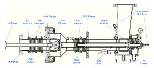
Figure 4.5.5: 2D section view of the injector input coupler.
