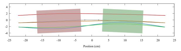
Figure 2.6.4: Periodic orbits in the arc cell. Also shown are the coordinate reference segments and the nominal magnet positions. The width of the magnets shown is equal to the pipe aperture in the mid-plane.
