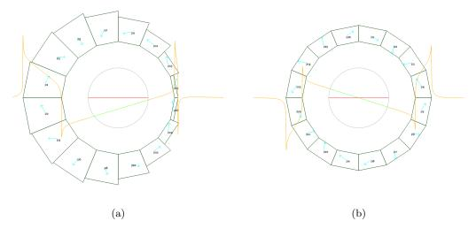
Figure 3.1.1: (Left) BD magnet. (Right) QF magnet. Orange graph is vertical field component  $B_y$  on the y=0 axis, with varying x position. The green segment is the field within the region required by the beams ( $\pm 23$ mm), which is meant to be linear. Magnetization axis is shown by blue arrows in each block.
