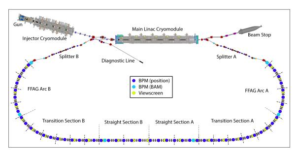
Figure 10.3.4: Beamline layout during full arc commissioning. The "flat pass" layout of the first splitter lines is shown, allowing energy recovery after a single pass.
