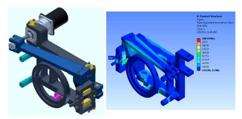
Figure 5.3.5: MLC cavity frequency tuner with fast piezoelectric actuators and increased stiffness for the main linac cavities. Left: CAD model. Right: ANSYS simulation of the von Mises stress for a tuning force of 26 kN applied to the cavity. The maximum stress is well below the yield strength of stainless steel at cryogenic temperatures.
