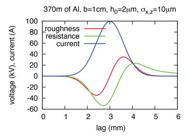
Figure 2.11.3: bunch current and induced voltage
