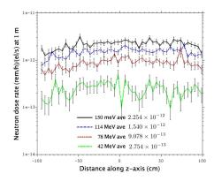
(a) Unshielded gamma dose rate at 1 m from(b) Unshielded neutron dose rate at 1 m from CBETA vacuum chamber.
