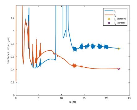
Figure 2.3.3: Transverse emittances through injector and main linac for 100 pC bunches.
