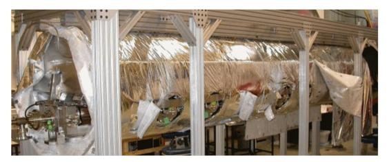
Figure 4.5.14: Photograph of the completed ERL injector 100 K shield being wrapped with MLI.
