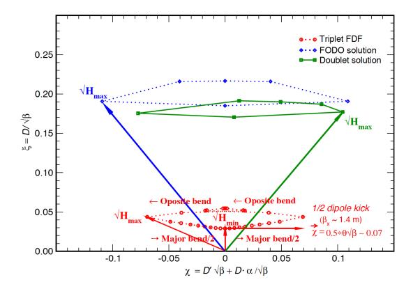
Figure 2.2.2: Normalized dispersion function for three basic cell configurations — triplet, FODO, and doublet – using the same magnets.
