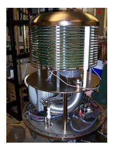
Figure 4.2.4: The HV section of the 750kV power supply. Individual circuit boards are visible inside the potential grading rings. The primary winding of the insulating core transformer is the large diameter gray-insulated wire below the circuit boards. The HV section is mounted in the pressurized  $SF_6$  tank with its axis parallel to the axis of the gun ceramic.
