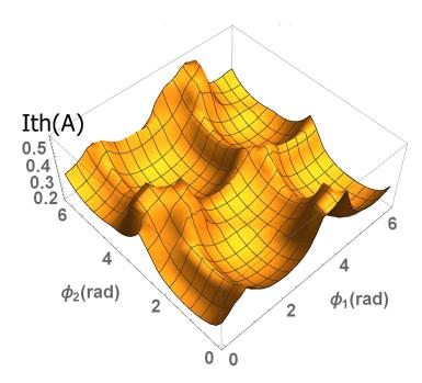
Figure 2.16.6: A scan of BBU  $I_{\rm th}$  over the two free phases for the CBETA 1-pass lattice with x-y coupling. Each cavity is assigned with a random set of 3 dipole HOMs in both x and y polarization. ( $\epsilon=125\,\mu{\rm m}$ ). For this particular HOM assignment,  $I_{\rm th}$  ranges from 140mA to 520mA.
