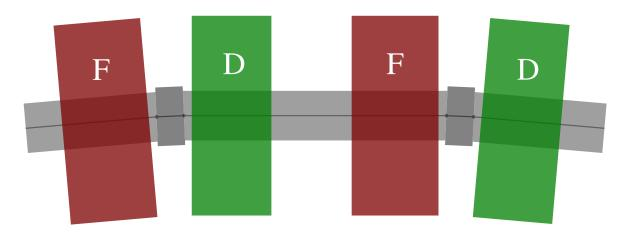
Figure 2.6.1: Illustration of FFAG arc cell geometry, showing two full cells. Lines show the reference geometry, with dots delimiting the ends of the segments. Magnet offsets are the distance of the magnet ends from the nearest dot. Segments bend by half the cell bend angle at each dot.
