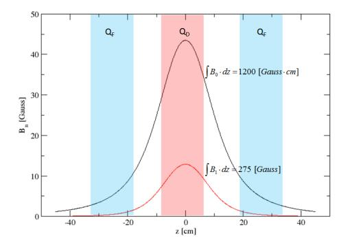
Figure 3.2.3: The black and red lines are the plots of the strengths of the dipole and quadrupole multipoles of the window frame magnet which surrounds the FFAG magnet (pink renctangle). The values of integrated strengths of these multipoles are 1200 [Gauss.cm] and 275 [Gauss]
