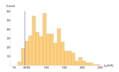
Figure 2.16.3: 500 BBU simulation results of  $I_{\rm th}$  for the CBETA 4-pass lattice. Each cavity is assigned with a random set of 10 dipole HOMs ( $\epsilon = 250\,\mu{\rm m}$ ). The blue line indicates the UPP of 40mA for the 4-pass machine.
