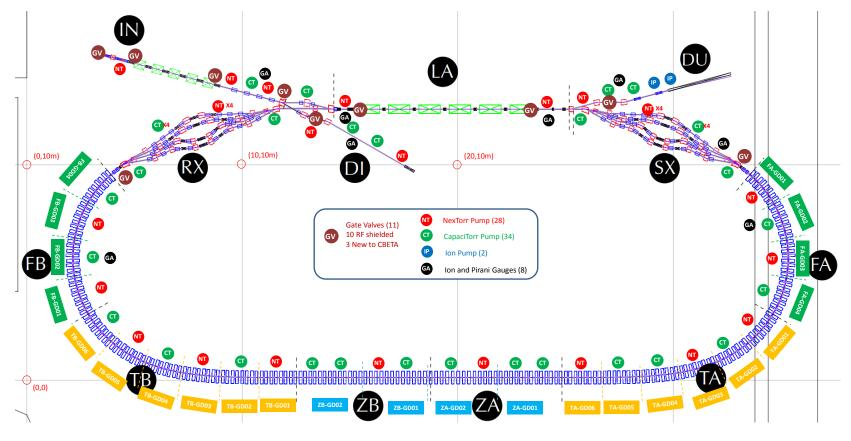
Figure 7.4.2: A proposed distribution of CBETA vacuum pump, gauges, and gate valves. Also shown are labels of FFAG girders, such as Girder 01 in FA section: FA-GD01.
