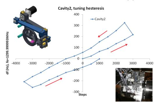
Figure 5.5.8: Result of testing of the course tuner driven by a stepper motor. The observed hysteresis of 150 Hz is as expected and will be compensated by the action of the fine tuner driven by piezo actuators.
