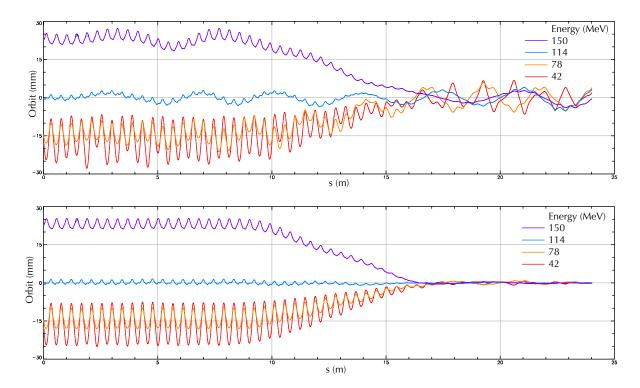
Figure 2.13.1: Example of simultaneous orbit correction for four beams with uniform horizontal and vertical offset errors in all FFAG magnets. Offsets are uniformly distributed within  $\pm 200\,\mu\text{m}$ . Every F quadrupole has a horizontal corrector, and every D quadrupole has a vertical corrector. BPMs are placed in the short drift between these magnets in each cell.
