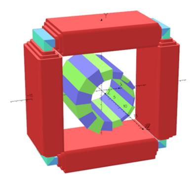
Figure 3.2.1: A window frame magnet with four coils (one coil in each side) can generates a normal quadrupole field, by connecting to a power supply in series the two outer layers of each of the four coils, and a normal dipole field by connecting in series to a power supply the innermost layer of the left and right coil, and a skew dipole by connecting in series to a power supply the innermost layer of the top and bottom coil.
