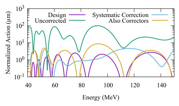
Figure 2.6.8:  $J_{\text{str}}(E)$  for TA. "Design" is for the hard edge model, and is the same as Fig. ??. "Uncorrected" is with field maps, when  $f_T$  alone is used to position the magnets. "Systematic Correction" applies an additional systematic correction to each magnet type as described in the text. "Also Correctors" additional applies correctors on the QF magnets in the transition to make  $J_{\text{str}}(E)$  be zero at the design energies.
