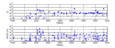
Figure 4.5.8: Simulated monopole mode damping in the full ERL injector (CLANS results). Top: Quality factor of all monopole modes between 1.5 GHz and 5.5 GHz. Bottom:  $R/Q \cdot Q$  of these modes. Realistic complex dielectric properties where used in these simulations for the RF absorbing materials in the HOM dampers.
