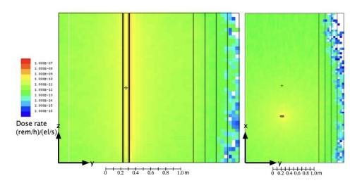
Figure 9.3.8: Neutron dose rate contours in the plane of the electron beam.
