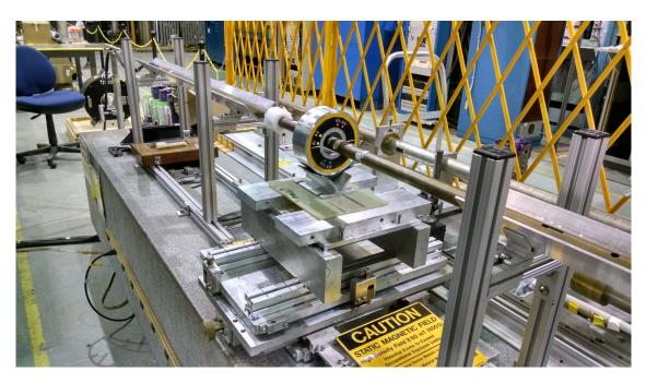
Figure 3.1.9: A prototype QF Halbach magnet being measured on BNL's rotating coil.
