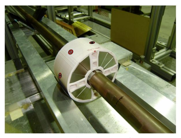
Figure 11.2.1: Harmonic coil measurements and magnet fiducialization.
