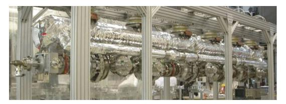
Figure 4.5.13: Beamline string hung from the GRP for the ERL injector .
