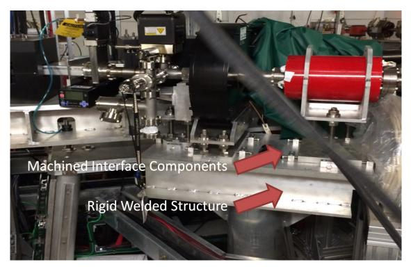
Figure 3.4.1: Welded structure.
