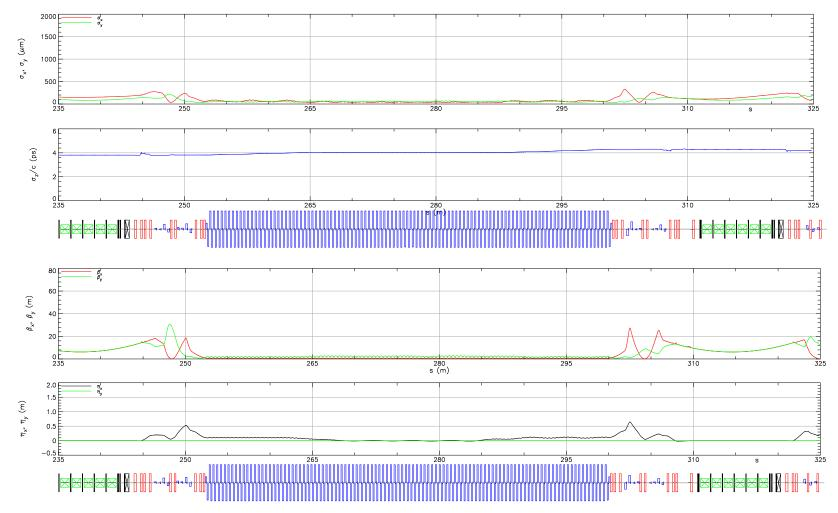
Figure 2.15.6: Optics and beam sizes for pass  $4,\,150~\mathrm{MeV}$
