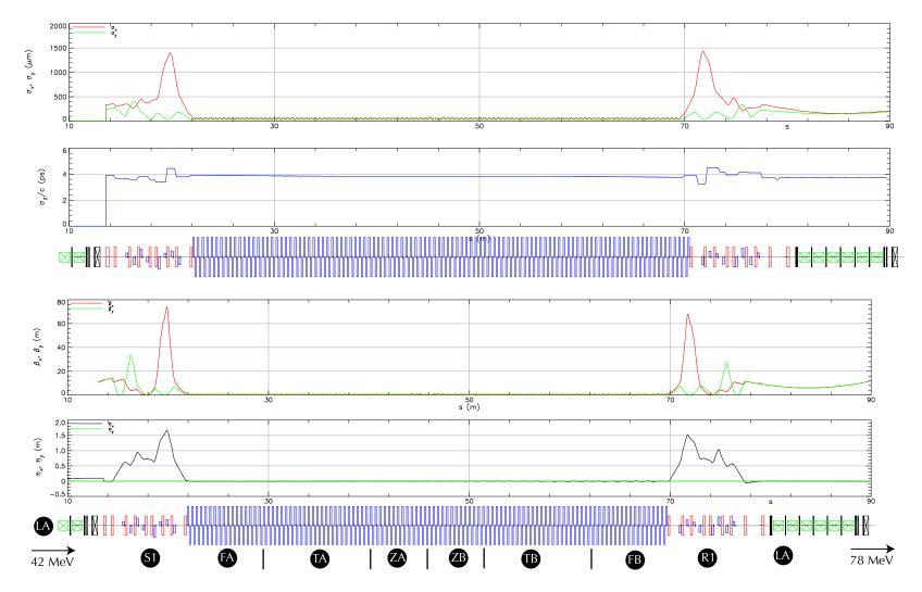
Figure 2.15.3: Optics and beam sizes for pass 1, 42 MeV
