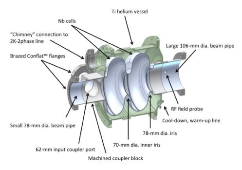
Figure 4.5.1: ERL injector cavity.
