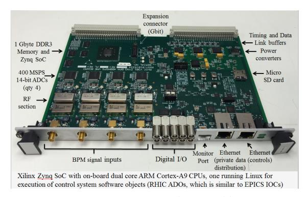
Figure 8.2.1: BNL V301 BPM electronics module
