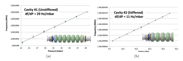
Figure 5.5.7: Tuning sensitivities of the unstiffened and the stiffened cavities.
