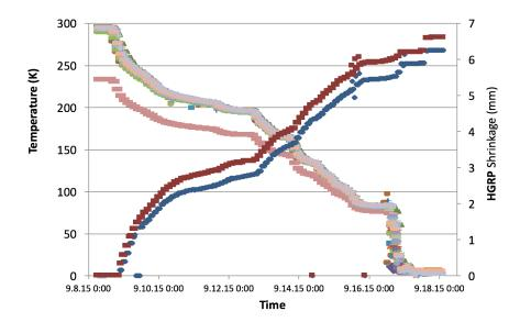
Figure 5.5.3: Movement of the outer (sliding) support posts: as the temperature of the HGRP goes down the posts move inwards. The movement was as expected.
