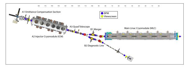
Figure 10.3.2: Beamline layout during MLC and diagnostic line commissioning. BPMs and viewscreens are highlighted with blue and yellow circles, respectively.
