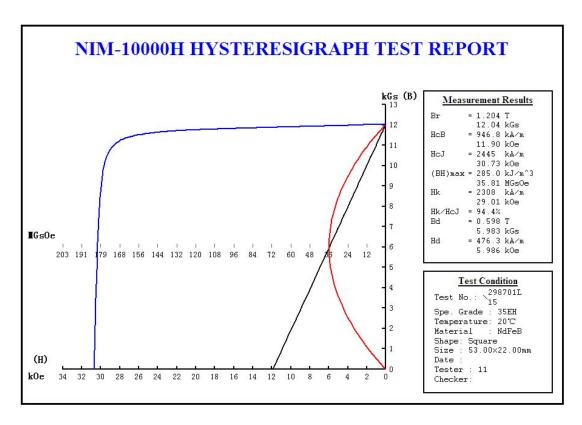
Figure 3.1.2: B-H curve of the AllStar Magnetics N35EH NdFeB permanent magnet material.
