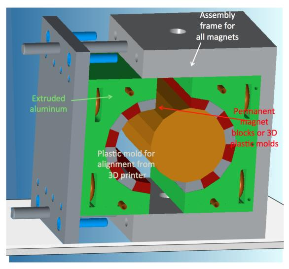
Figure 3.3.3: Assembly procedure starts with the 3D mold built with plastic but using an aluminum future made for all magnets.
