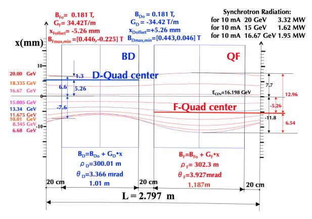
Figure 2.2.3: Orbits and dimensions of the eRHIC NS-FFAG basic arc cell.
