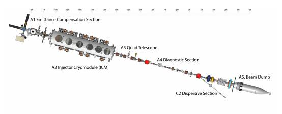
Figure 4.1.1: A schematic of the Cornell photoinjector after installation and recommissioning for use in CBETA.
