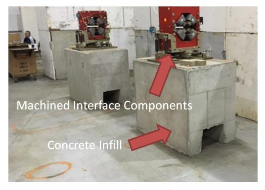
Figure 3.4.3: Concrete infill.
