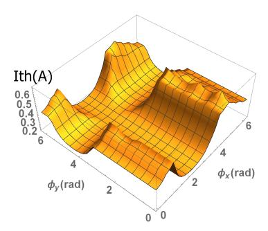
Figure 2.16.4: A scan of BBU  $I_{\rm th}$  over the two phase advances for the CBETA 1-pass lattice. Each cavity is assigned with a random set of 3 dipole HOMs in both x and y polarization. ( $\epsilon = 125\,\mu{\rm m}$ ). For this particular HOM assignment,  $I_{\rm th}$  ranges from 140mA to 610mA.
