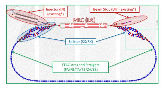
Figure 7.1.1: CBETA Layout and vacuum sections.
