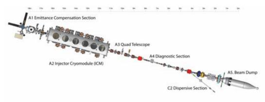
Figure 4.1.1: A schematic of the Cornell photoinjector after installation and recommissioning for use in CBETA.
