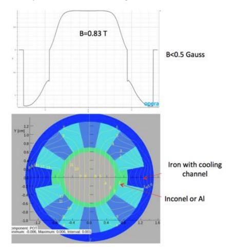
Figure 2.7.3: Preliminary design of the Halbach extraction dipole. (Courtesy of N. Tsoupas).
