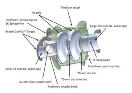
Figure 4.5.1: ERL injector cavity.
