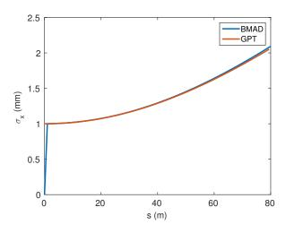
Figure 2.10.1: Comparison of Bmad and GPT space charge models for a drifting 42 MeV Gaussian beam.
