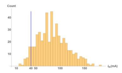
Figure 2.16.2: 500 BBU simulation results of  $I_{\rm th}$  for the CBETA 4-pass lattice. Each cavity is assigned with a random set of 10 dipole HOMs ( $\epsilon = 125 \,\mu{\rm m}$ ). The blue line indicates the UPP of 40mA for 4-pass machine.
