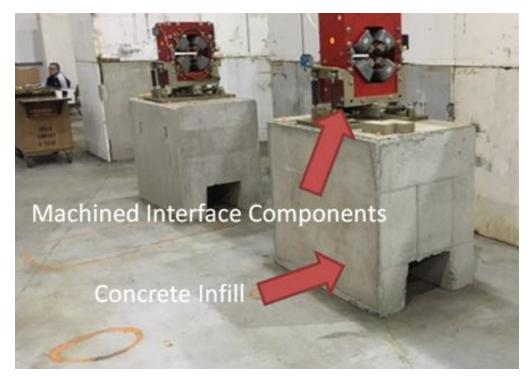
Figure 3.4.3: Concrete infill.
