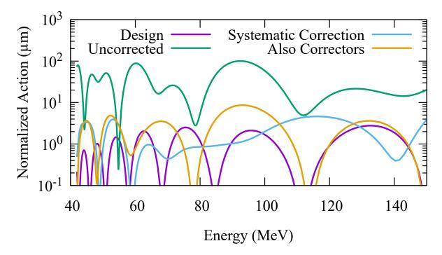
Figure 2.6.8:  $J_{\text{str}}(E)$  for TA. "Design" is for the hard edge model, and is the same as Fig. ??. "Uncorrected" is with field maps, when  $f_T$  alone is used to position the magnets. "Systematic Correction" applies an additional systematic correction to each magnet type as described in the text. "Also Correctors" additional applies correctors on the QF magnets in the transition to make  $J_{\text{str}}(E)$  be zero at the design energies.
