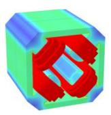
Figure 2.5.4: Color contours of the modeled field magnitude on the steel surface of the quadrupole magnet at 4.9 T/m excitation. The field ranges up to 13.0 kG (red) on the end corners of the pole.
