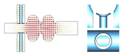
Figure 4.5.2: Geometry of the cavity and details of the coupler antenna with the electric field lines of the fundamental mode indicated
