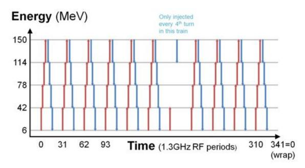
Figure 2.8.1: Bunch pattern produced in the eRHIC-like mode that has a circumference of h = 343 RF wavelengths but a time periodicity of 341 RF periods.
