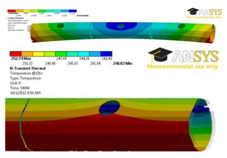
Figure 5.4.3: Cool-down analysis of the thermal shield (Aluminum). As it is cooled only on one side, the cool-down will not be uniform, resulting in an up to 13K temperature difference (a) and a lateral bending of up to 6 mm (b).
