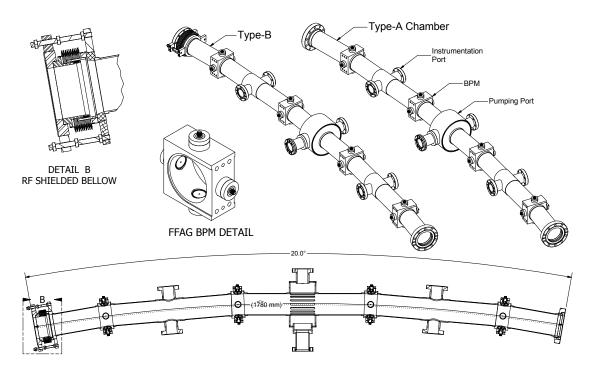
Figure 7.3.1: A FFAG arc 4-cell beam pipe design. The 1.78 m long beam pipe assembly houses 4 sets of 4-button BPMs on the 7 cm drifts between QF and QD magnets. One pump port and two beam instrumentation ports are on the 12 cm middle drifts between FFAG cells.
