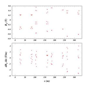
Figure 2.5.3: Distributions of required splitter dipole and quadrupole magnet field strengths versus the longitudinal orbit coordinate s. The magnets are thus ordered from left to right S1-R1-S2-R2-S3-R3-S4-R4.
