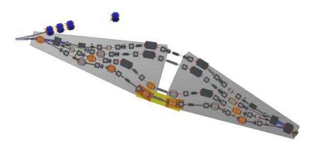
Figure 2.5.9: Placement of the H-dipole (dark gray) and quadrupole (light gray) magnets in the SX region. Four vertical corrector magnets are shown (blue) to exemplify how the space constraints can be satisfied. The magnet shown in purple on the upper left is one of the four septum magnets under design. The bellows in the S1 line shows how the path length adjustment for energy recovery is achieved.
