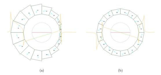
Figure 3.1.1: (Left) BD magnet. (Right) QF magnet. Orange graph is vertical field component  $B_y$  on the y=0 axis, with varying x position. The green segment is the field within the region required by the beams (±23mm), which is meant to be linear. Magnetization axis is shown by blue arrows in each block.
