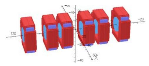
Figure 3.2.2: Isometric view of six of the permanent magnets of the CBETA arc.
