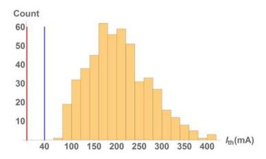
Figure 2.16.1: 500 BBU simulation results of  $I_{\rm th}$  for the CBETA 1-pass lattice. Each cavity is assigned with a random set of 10 dipole HOMs ( $\epsilon = 125 \,\mu{\rm m}$ ). The red line indicates the KPP of 1mA, while the blue line indicates the UPP 40mA for 1-pass machine.
