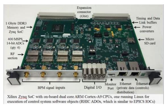
Figure 8.2.1: BNL V301 BPM electronics module
