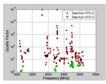
Figure 5.3.7: External Quality factor of the Cornell 7-cell ERL cavity without (red) and with (green) HOM absorbers installed.
