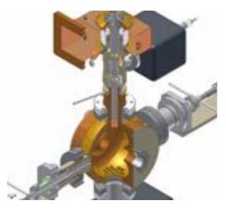
Figure 4.4.1: 3D view of the buncher cavity showing input coupler, plunger-type frequency tuner, pumping slots.
