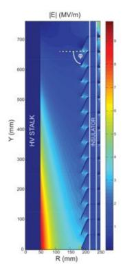
Figure 4.2.2: Simplified HV model made in the software Opera 2D. Shown is the HV stalk, insulator, and guard rings for the gun operating at 750 kV. Color corresponds to the magnitude of the electric field in MV/m. For simplicity, this HV model is monolithic, rather than made of two insulator assemblies (as built), and similarly does not show the triple point protection rings.
