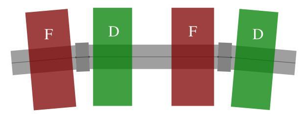
Figure 2.6.1: Illustration of FFAG arc cell geometry, showing two full cells. Lines show the reference geometry, with dots delimiting the ends of the segments. Magnet offsets are the distance of the magnet ends from the nearest dot. Segments bend by half the cell bend angle at each dot.
