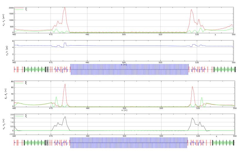
Figure 2.15.9: Optics and beam sizes for pass 7, 42 MeV
