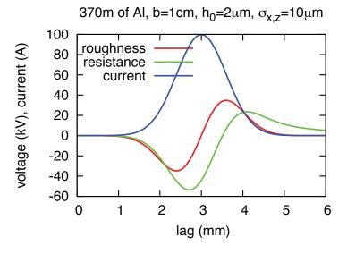
Figure 2.11.3: bunch current and induced voltage
