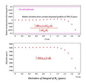
Figure 2.5.5: The upper plot shows the relative deviation of the field gradient integral from that of the perfectly uniform case. The lower plot shows the variation of the field gradient integral. The  $10^{-4}$  specification is satisfied over 30 mm of the 34-mm width of the vacuum chamber.
