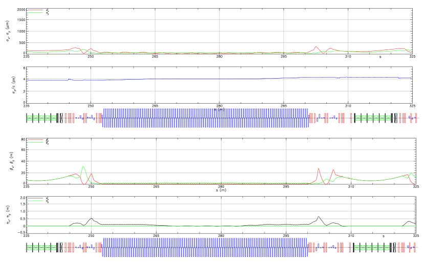
Figure 2.15.6: Optics and beam sizes for pass 4, 150 MeV
