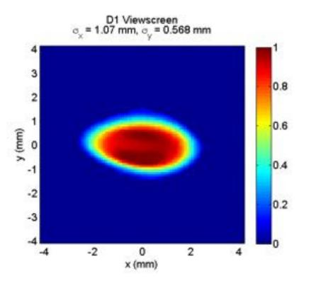
Figure 1.6.1: The first beam accelerated by the MLC, captured on a viewscreen directly after the MLC.
