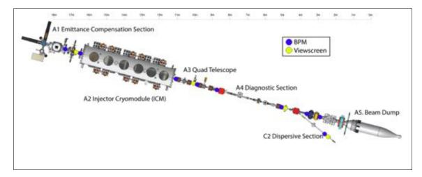
Figure 10.3.1: Beamline layout during gun-linac-dump recommissioning. BPMs and viewscreens are highlighted with blue and yellow circles, respectively.
