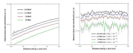
(a) Unshielded gamma dose rate at 1 m from(b) Unshielded neutron dose rate at 1 m from CBETA vacuum chamber. CBETA vacuum chamber.
