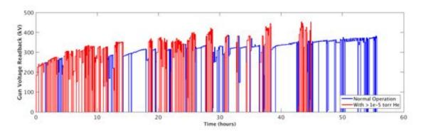
Figure 4.2.5: The voltage applied to the gun during conditioning. Data points are colored for UHV (blue dot) and helium (red) conditioning.
