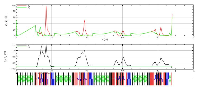
Figure 2.5.2: Optics in SX and LA for the first four accelerating passes, including a short piece of the FA beamline following each SX line. Remaining FFAG beamline and RX are omitted.
