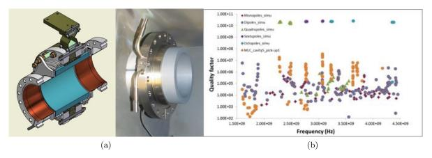
Figure 5.5.6: Performance of the higher order mode absorber. On the left a schematic view of the absorber is given, where is absorbing material (a SiC composite) is shown in blue. The absorbing cylinder is pictured in the center. On the right, the measured quality factors of some higher order modes, compared to undamped resonances are given showing that the absorber operates as designed.
