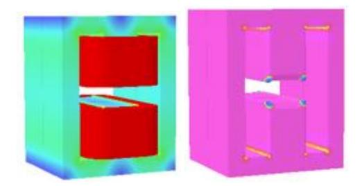
Figure 2.5.6: Color contours of the modeled field magnitude on the steel surface of the 20-cmlong dipole magnet models (left) and of the magnetic permeability (right). The field values ranges up to 18 kG (red) in the return yoke for the central field value of 3.8 kG. The magnetic permeability value ranges from 2.4 (blue) to 10<sup>4</sup> (pink).
