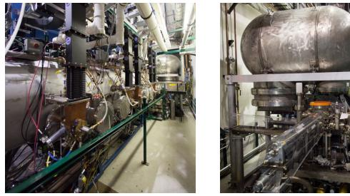
(a) Injector cryomodule
