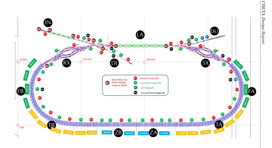
Figure 7.4.2: A proposed distribution of CBETA vacuum pump, gauges, and gate valves. Also shown are labels of FFAG girders, such as Girder 01 in FA section: FA-GD01.
