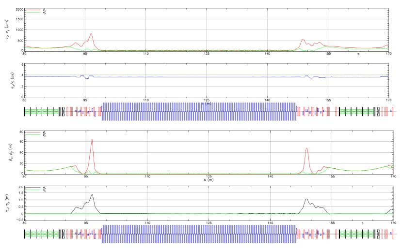
Figure 2.15.4: Optics and beam sizes for pass 2, 78 MeV
