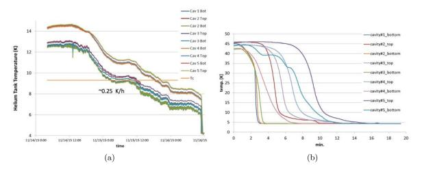
Figure 5.5.4: Slow (left) and fast (right) cool-down cycle performed in order to measure cycle dependent impacts on the cavity performance. For the slow cool-down we were able to get 0.25 K/h while the fast cool-down resulted in 0.5 K/min – 2 K/min, depending on how close the cavity was to the JT valve.
