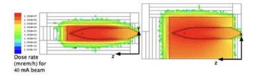
Figure 9.3.4: Gamma dose rate contours in mrem/h or a 6 MeV, 40 mA electron beam.
