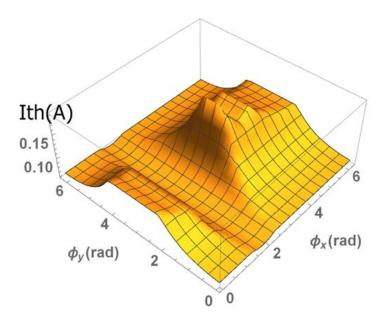
Figure 2.16.5: A scan of BBU  $I_{\rm th}$  over the two phase advances for the CBETA 4-pass lattice. Each cavity is assigned with a random set of 3 dipole HOMs in both x and y polarization. ( $\epsilon = 125 \,\mu {\rm m}$ ). For this particular HOM assignment,  $I_{\rm th}$  ranges from 61mA to 193mA.
