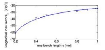
Figure 4.5.7: Total loss factor in the injector cryomodule beamline with 5 2-cell cavities as a function of bunch length.
