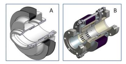
Figure 7.3.5: RF shielded belows used in CESR (A) and in Cornell Prototype injector (B).
