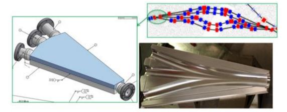
Figure 7.3.4: Example design for beam splitting and combing chamber, by welding two machined aluminum halves with smooth beam path transitions.
