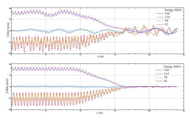
Figure 2.13.1: Example of simultaneous orbit correction for four beams with uniform horizontal and vertical offset errors in all FFAG magnets. Offsets are uniformly distributed within  $\pm 200 \,\mu$ m. Every F quadrupole has a horizontal corrector, and every D quadrupole has a vertical corrector. BPMs are placed in the short drift between these magnets in each cell.
