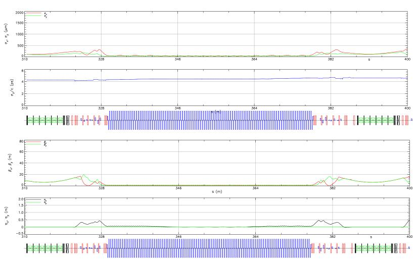
Figure 2.15.7: Optics and beam sizes for pass 5, 114 MeV
