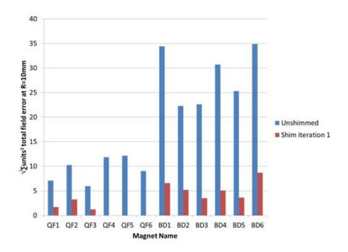
Figure 3.1.10: The quadrature sum of higher harmonic units  $\sqrt{\sum_{n=3}^{15} a_n^2 + b_n^2}$  in the Halbach prototypes, converted to R=10mm for comparison (because only the smaller coil size would fit through the BD magnet aperture).
