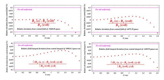
Figure 2.5.7: Modeled field uniformity for the H-dipole magnet designs. The upper plots show the relative deviation of the field from the central field value in the middle of the magnet. The lower plots show the relative deviation of the field integral from the ideal case. Left: 20-cm-long model at 3.8 kG central field strength. Right: 30-cm-long model at 4.5 kG central field strength.
