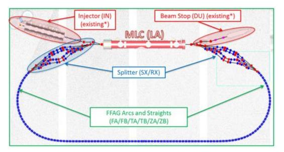
Figure 7.1.1: CBETA Layout and vacuum sections.
