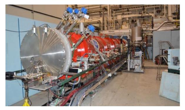
Figure 5.1.1: The Cornell Main Linac Cryomodule (MLC) installed for RF testing at Cornell.
