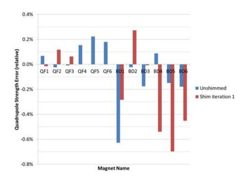
Figure 3.1.12: Error in the quadrupole strength of each magnet. This is potentially affected by temperature variation via the NdFeB temperature coefficient of  $-1.1 \times 10^{-3}$ /K.
