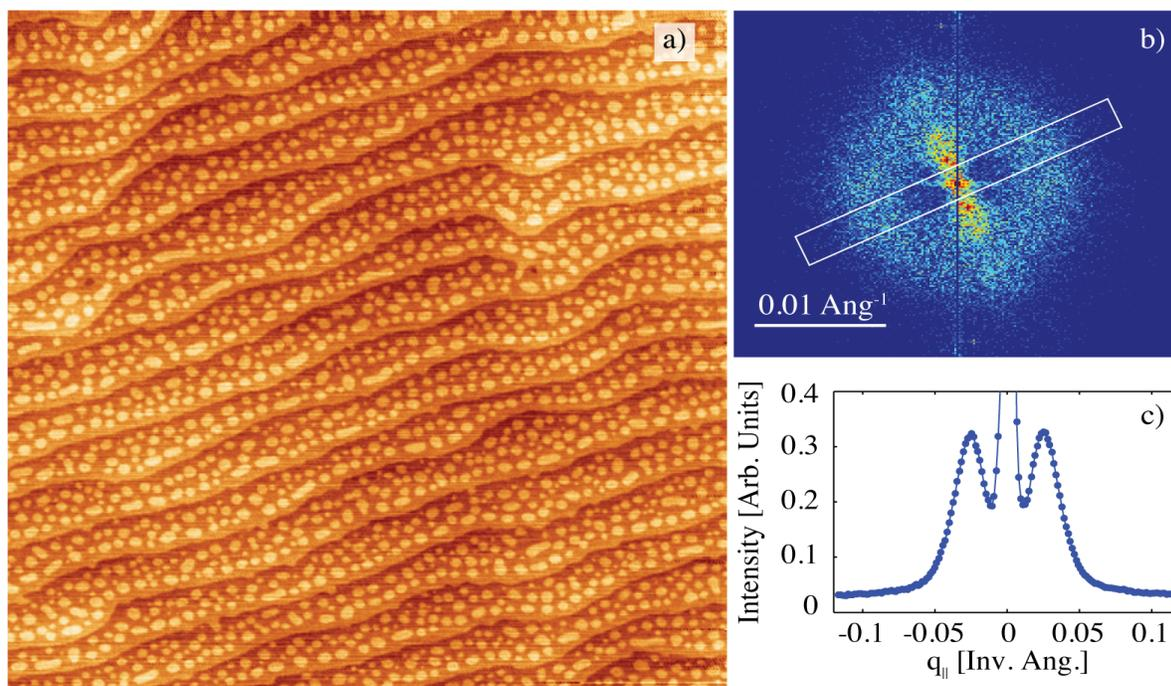
Figure 1.2.4: a) Atomic force microscope image of  $\langle 001 \rangle$  SrTiO<sub>3</sub> after pulsed-laser-deposition growth of 11.3 layers of SrTiO<sub>3</sub>. b) Fourier transformation of the AFM image, illustrating speckle in the diffuse ‘Henzler rings’ associated with the island structure. c) Diffuse scattering profile corresponding to the rectangular region in b, experimentally measured with an incoherent beam [44].
