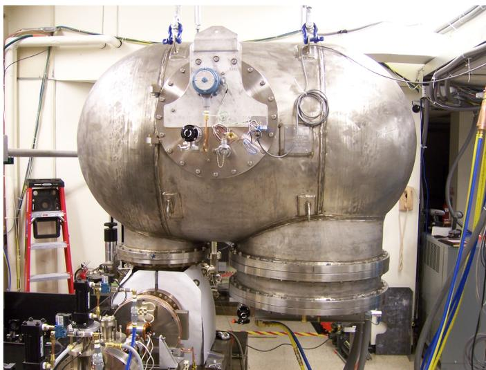
Figure 2.3.5: The Cornell gun with its SF<sub>6</sub> pressure vessel mounted. The HV power supply is mounted in the port to the right of the gun.
