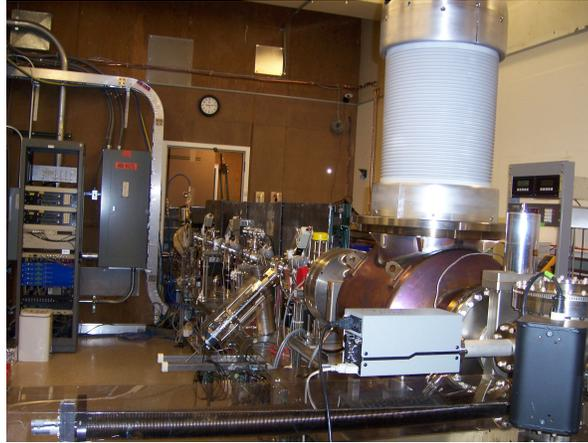
Figure 2.3.4: The developmental gun at Cornell, without its HV power supply and SF<sub>6</sub> tank, followed by the initial test beamline. The load-lock system is on the right rear of the gun.
