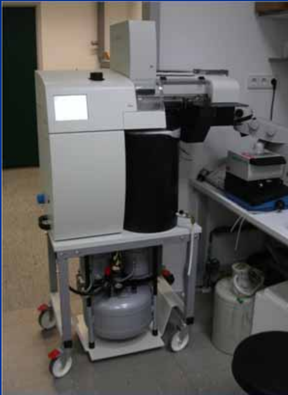
Leica EM-PACT2 high pressure freezing machine (2.5 kbar)
