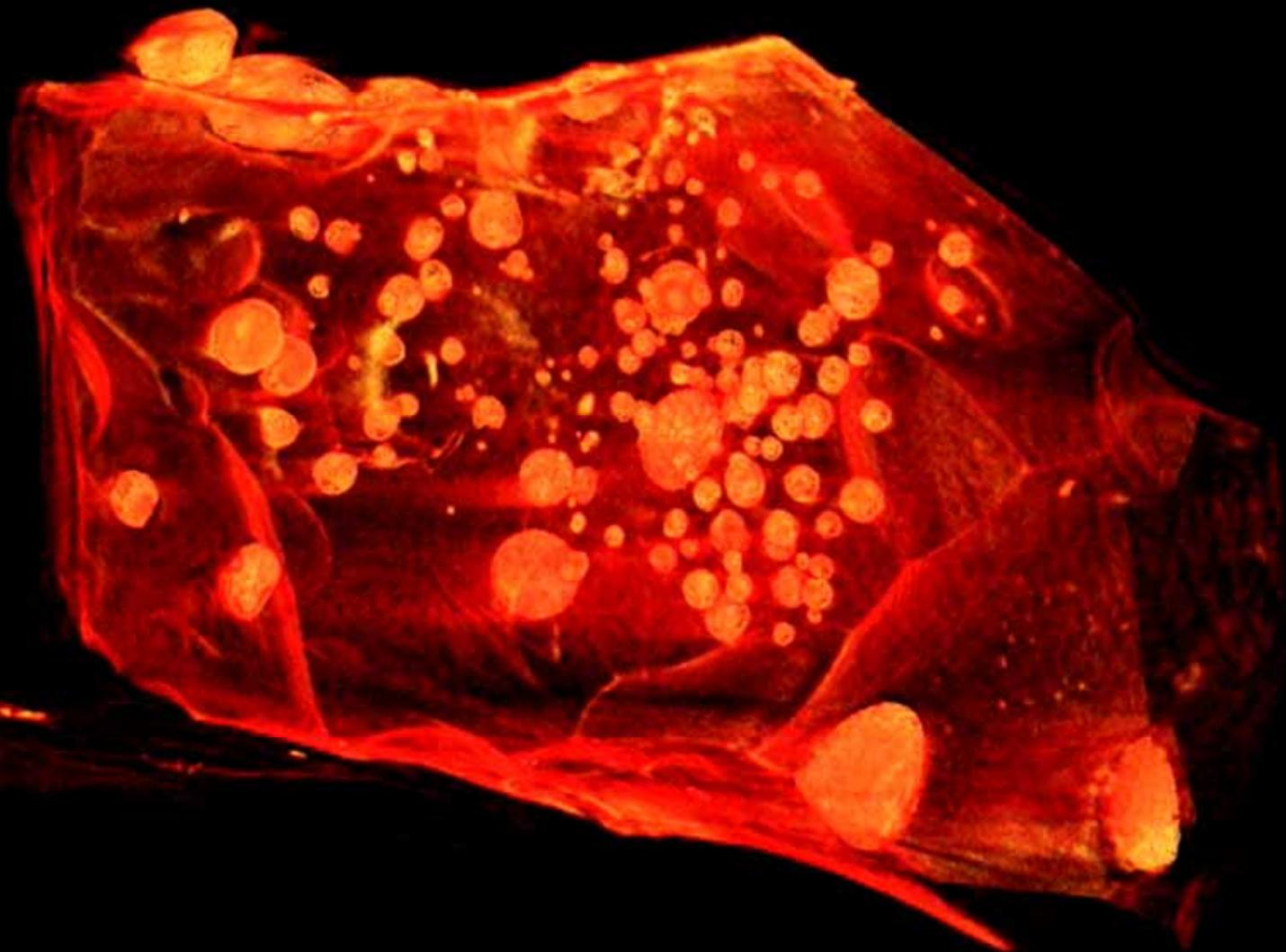
Fe+10wt%S spheres within a SC olivine,  $(\text{Mg}_{0.88}\text{Fe}_{0.12})_2\text{SiO}_4$
