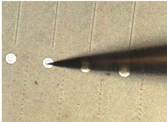
**Figure C.18:** Photograph under microscope of the probe making contact with a sensor input pad.
