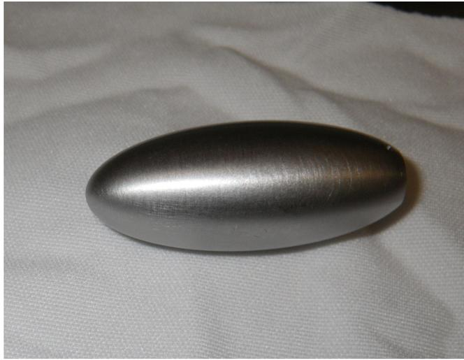
Figure 7.35: Ellipsoidal sample used to measure  $H_{c1}$  of  $\text{Nb}_3\text{Sn}$  coating using  $\mu$ -SR at TRIUMF.
