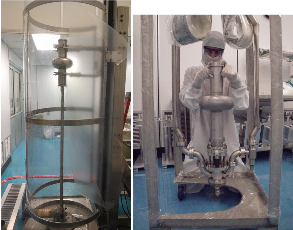
Figure 6.1: High pressure rinsing (left) and assembly of the cavity to the test stand (right).
