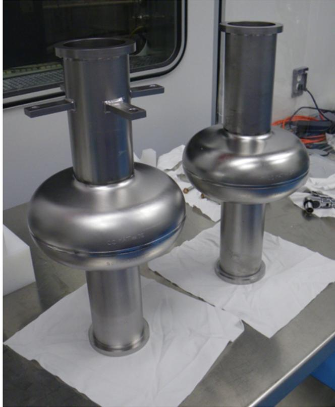
Figure 5.6: A  $\text{Nb}_3\text{Sn}$  cavity (left) stands next to an uncoated cavity.
