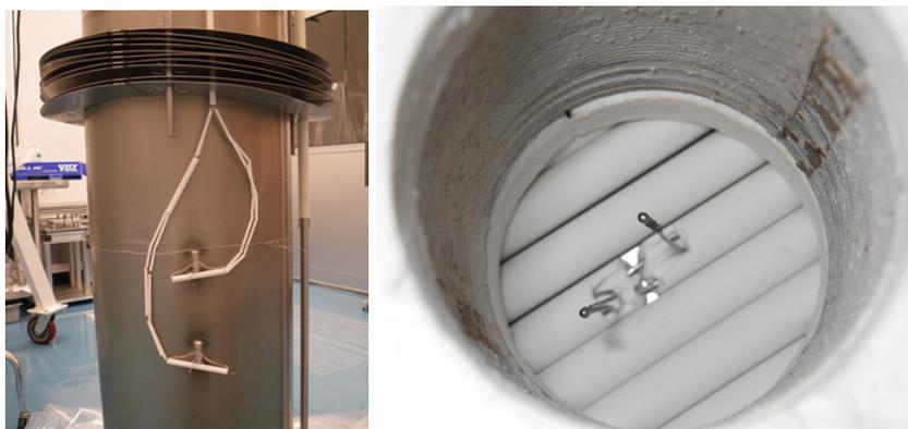
Figure 5.2: Thermocouples measuring the cavity temperature (left) and the tin source temperature (right).
