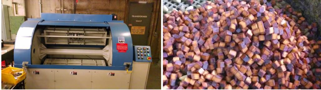
Figure 7.20: Centrifugal barrel polish machine loaded with Nb<sub>3</sub>Sn cavity (left); and polishing media after 4.5 hours (right).
