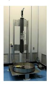
Figure 3: New high-pressure water rinsing system.
